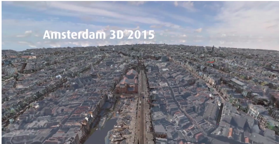
Figure 1.2: Multi view stereo mesh of city of Amsterdam : Amsterdam 3D (CycloMedia Technology, Inc)
