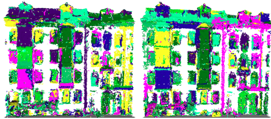
(a) Test data I region growing without texture information (b) Test data I region growing with texture information
