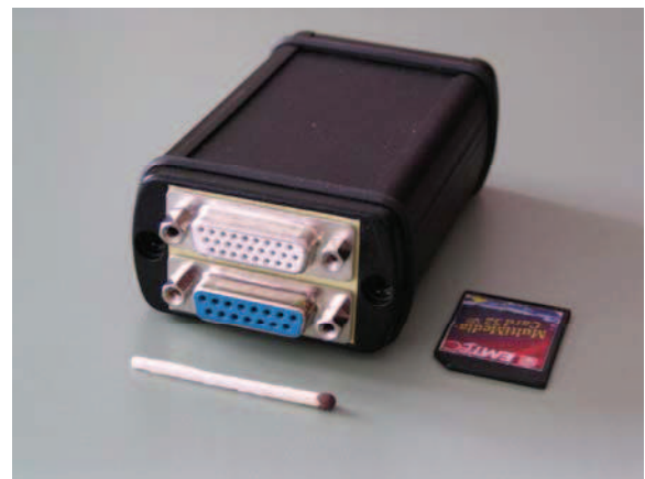
Figure 1: PRP-J5 flight data recorder placed into container housing.
