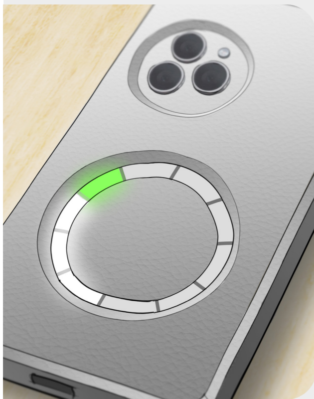
Figure 5.7. The Ring as it is executed on the smartphone. The first segment starts to light on the bottom left of the Ring, after the first month of ownership. It starts at the bottom to make a reference to the speedometer of a car.
