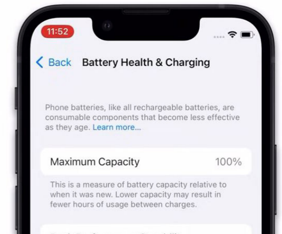
Figure 3.5. Apple's recent iPhone models indicate the maximum capacity of the battery, allowing the user to track its degradation (image from Proper Honest Tech, 2023).
