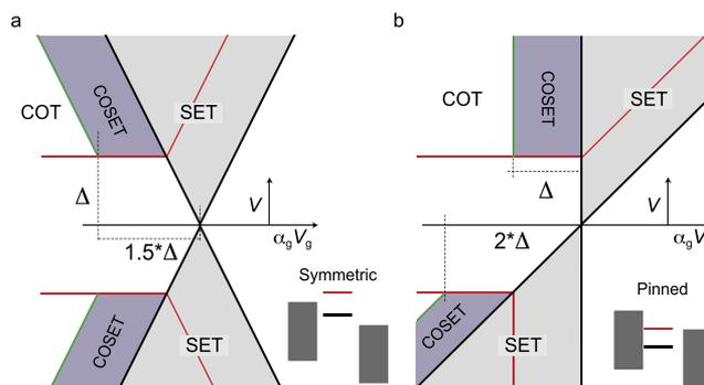
FIG. 16. How far is “off-resonant”? (a) Energy-energy stability diagram for symmetric capacitive coupling ( $C_L = C_R \gg C_g$ ) characteristic of molecular QD devices. (b) Strongly asymmetric couplings ( $C_L \gg C_R$ ). This is typical for molecular STM junctions, where the energy levels pin to one electrode (substrate), leaving the tip electrode to act as a probe. In this case, the energy  $\alpha_g V_g$  represents the *level equationment* with the Fermi-energy.
