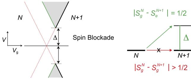
FIG. 10. SET spectroscopy of a high-spin molecule: spin blockade. If ground state transitions are spin-forbidden,  $|S_g^{N+1} - S_g^N| > 1/2$ , then the SET transport is suppressed (red dashed cross). Transport sets in only when a finite bias makes the lowest spin-compatible excitation energetically accessible. This can be either an  $N + 1$  state with  $|S_e^{N+1} - S_g^N| = 1/2$  (shown) or an  $N$  electron state with  $|S_g^{N+1} - S_e^N| = 1/2$  (not shown).
