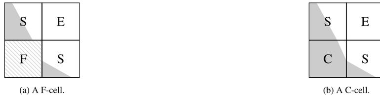
**Fig. 2.** Difference in labeling between F-cells (left) and C-cells (right). The gray area represents the geometrical reconstruction based on the fill ratio of the cells. Fluid is indicated by ■. The F-cell is not reconstructed and therefore illustrated with a hatched pattern representing a mixture of liquid and gas. New are the C-cells in which the free surface is reconstructed for a smoother interface between fluids.
