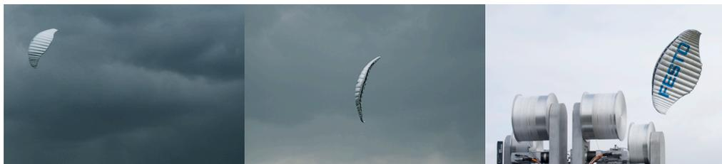
**Figure A.1** | Early generation quad-tether ram-air kites developed in collaboration with FESTO (circa 2010) [181].
