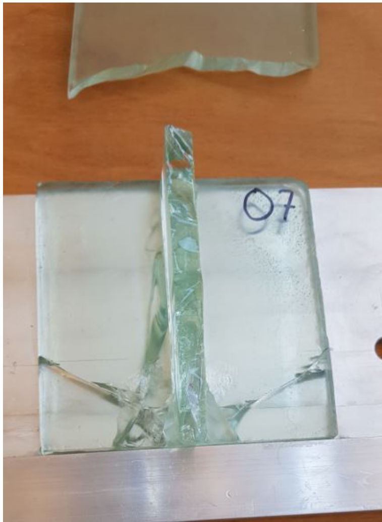
Figure E.7: Cracks in Specimen 7
