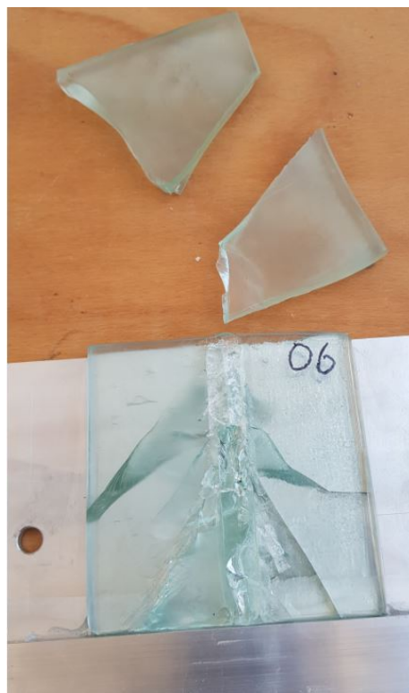
Figure E.6: Cracks in Specimen 6
