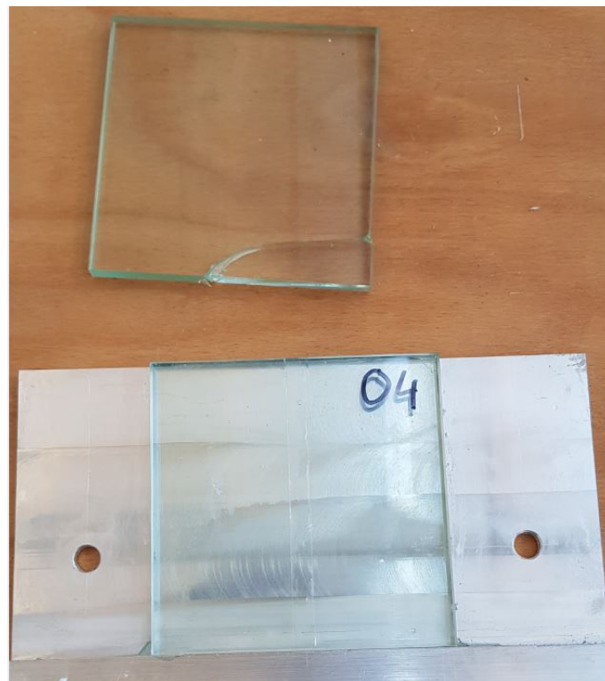
Figure E.4: Cracks in Specimen 4
