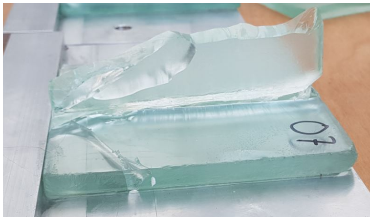
Figure E.8: Cracks in Specimen 7, side view
