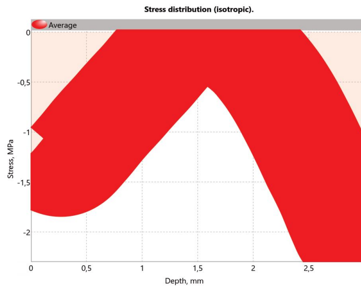
Figure C.4: SCALP Result Output for the remains of the web of specimen 11, near the weld
