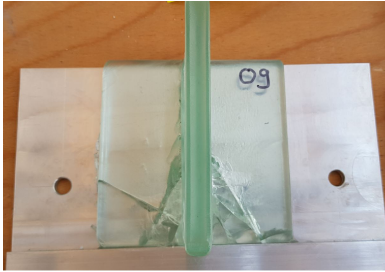
Figure E.11: Cracks in Specimen 9
