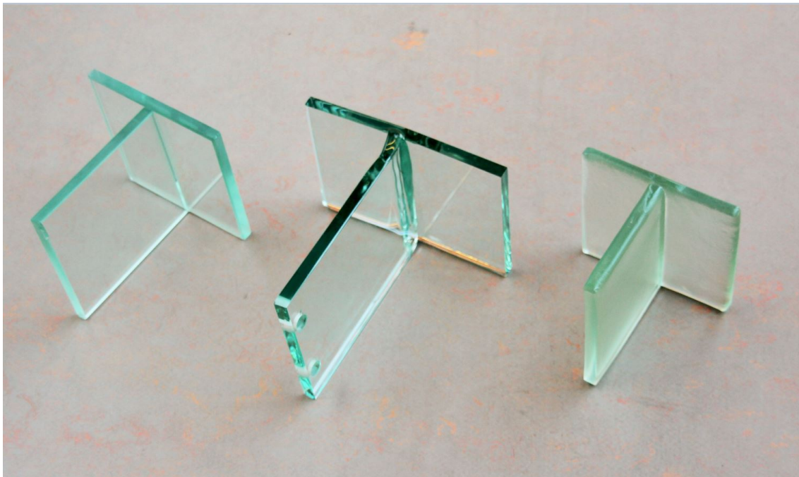
Figure 98: Adhesive (left), welded (center) and fused (right) objects.
