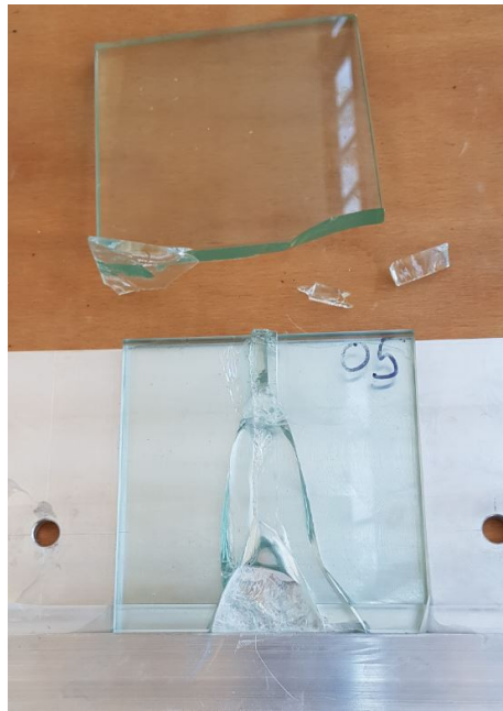
Figure E.5: Cracks in Specimen 5
