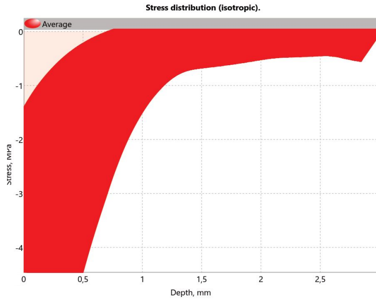
Figure C.2: SCALP Result Output for the remains of the web of specimen 10, near the weld
