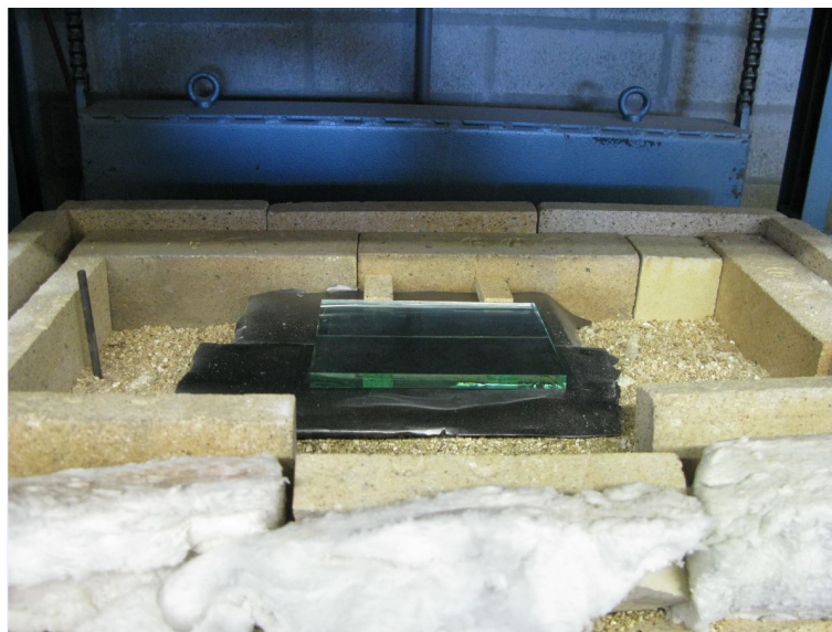
Figure 53: Positioning of the flange on the base of the oven prior to pre-heating. The ring of bricks closes the oven. The smaller ring on top is to be removed.
