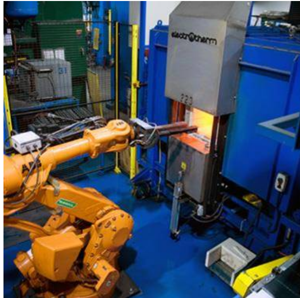
Figure 101: Robotic arm operating in oven (Electrotherm Electrical & Metal Products Ltd. 2018)
