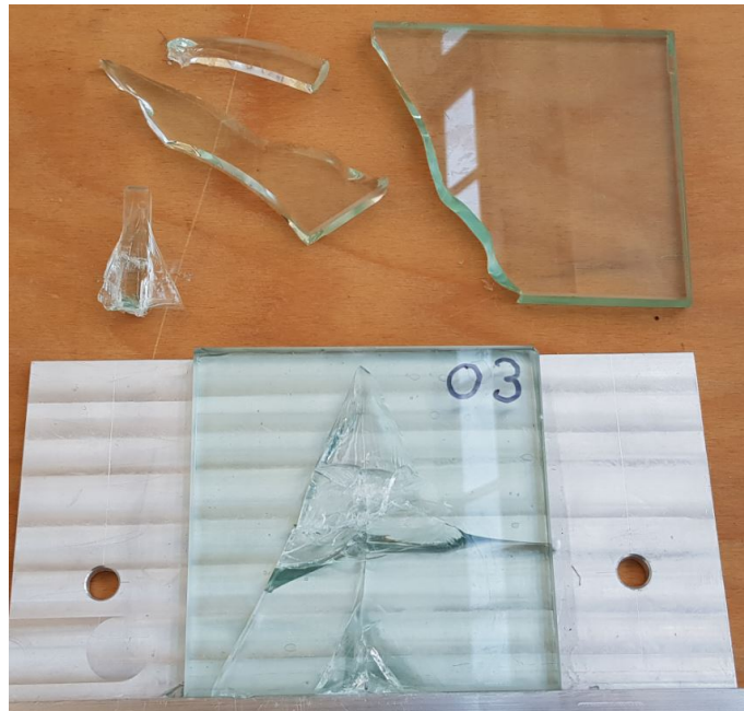
Figure E.3: Cracks in Specimen 3
