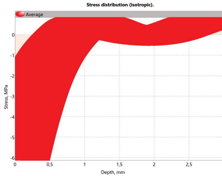
Figure C.1: SCALP Result Output for the remains of the web of specimen 10, between the holes
