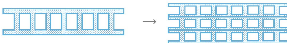
Figure 39: Design Example of the sandwichpanel with overdimensioning and secondary load transfer mechanisms
