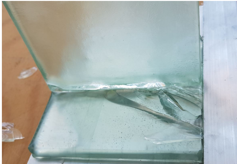
Figure E.10: Cracks in Specimen 8, side view
