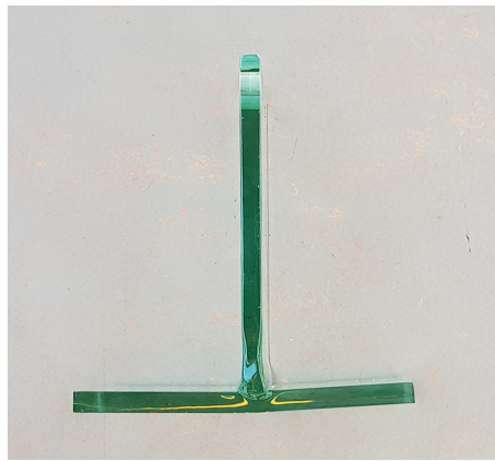
Figure 57: Welded specimen of first experiment, note the bent flange.
