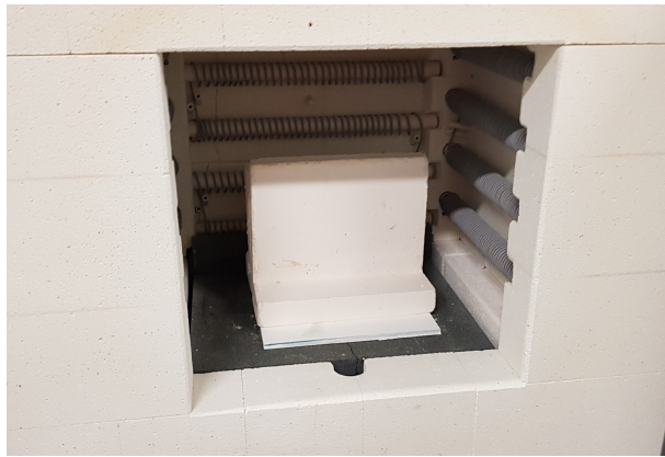
Figure 74: The moulds in position before experiment four. The base plate is a ceramic tile and no bricks were used for support.
