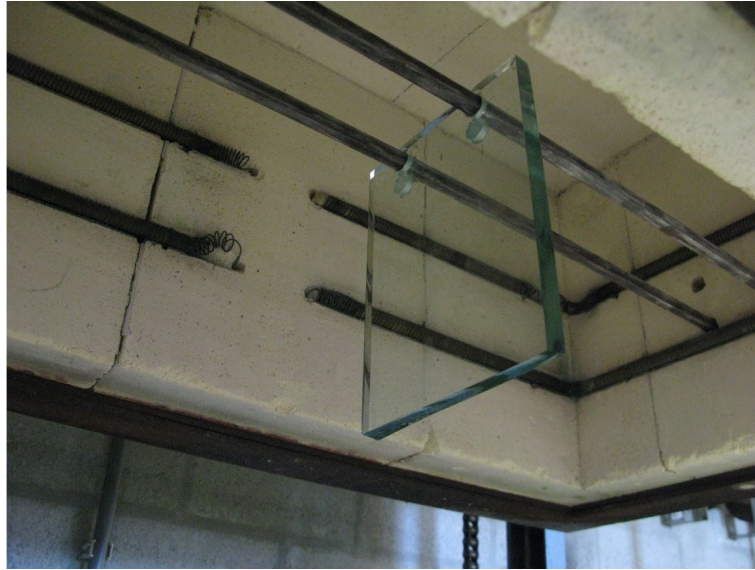
Figure 54: Suspension of the web on steel rods attached to the oven's box, prior to pre-heating.
