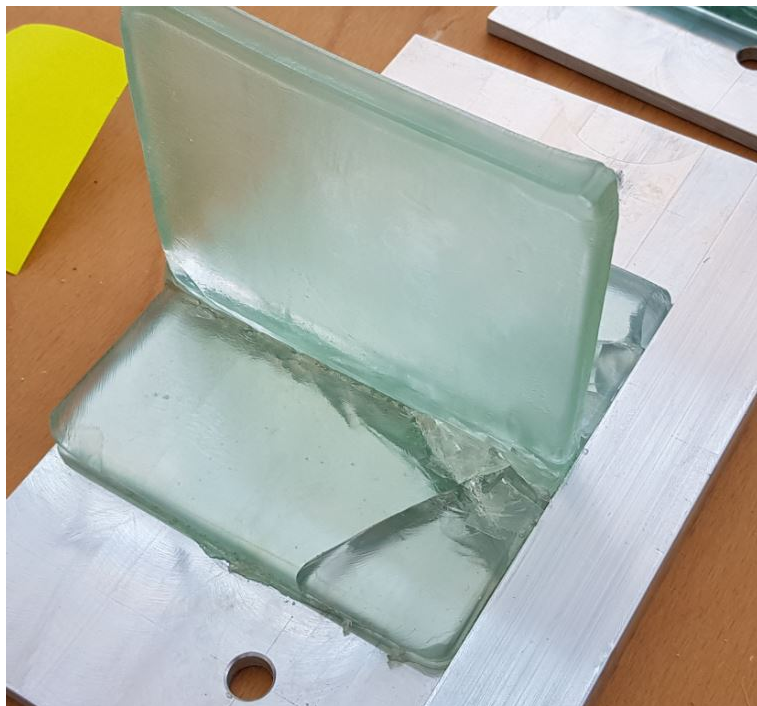
Figure E.12: Cracks in Specimen 9, side view
