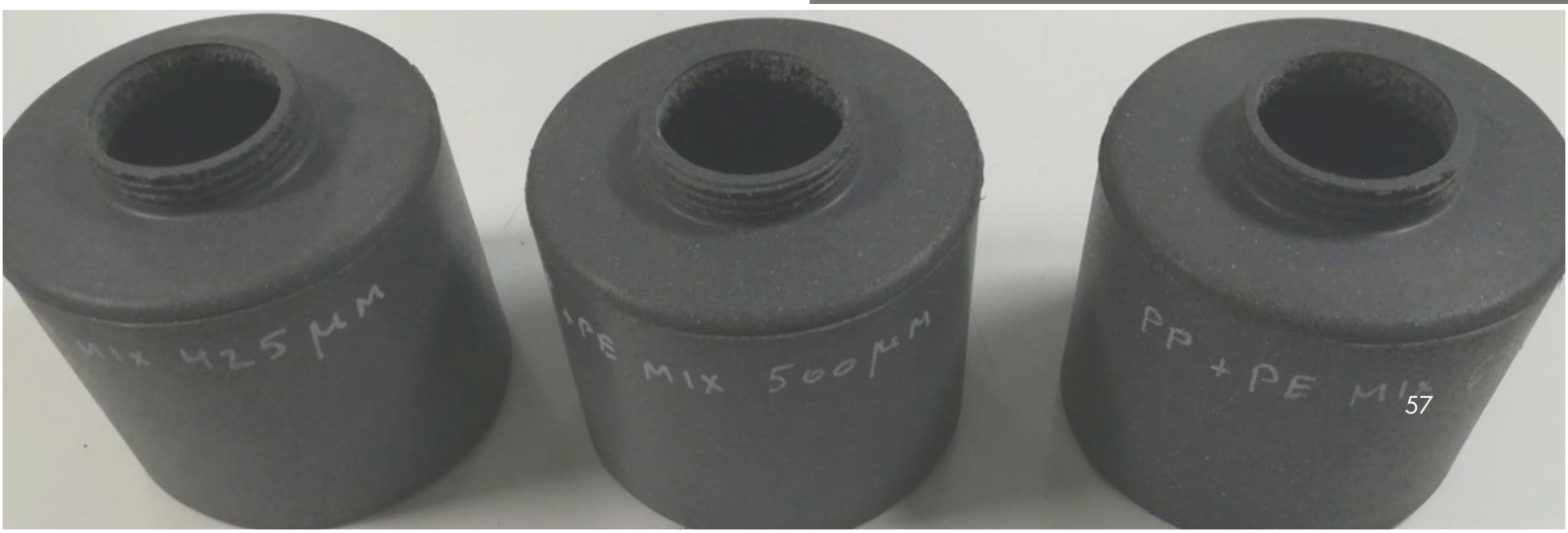
Figure 4.12 Tests with the powder produced at Maag, left 425 microns, middle 500 microns and right 630 microns.
