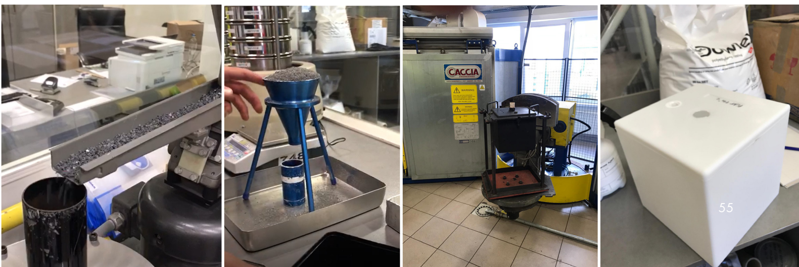
Figure 4.7 From left to right, making powder, measuring the dryflow, test setup and first test with virgin material
