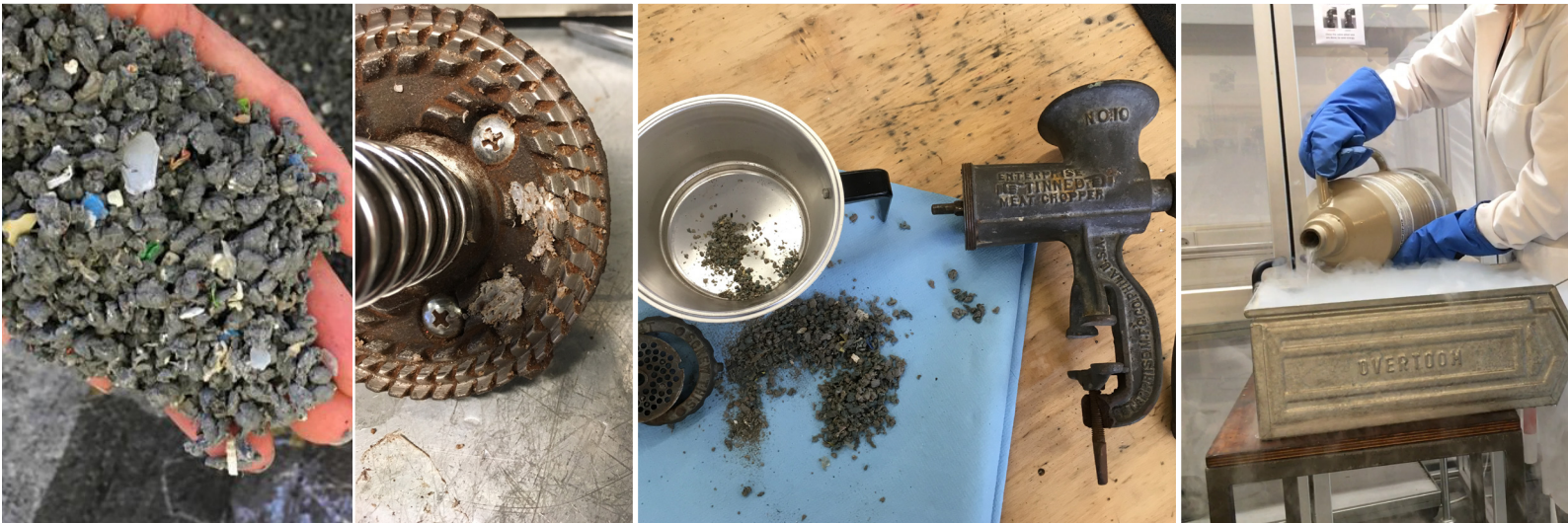
Figure 4.11 From left to right: the testing material PO95 agglomerate, melted plastic in the coffee grinder, and the meat grinder with a some shredded agglomerate.
