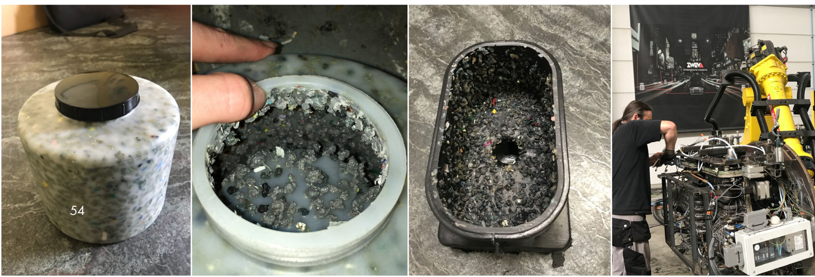
Figure 4.5 The first test with non powdered agglomerate together with virgin material into existing moulds of Zweva
