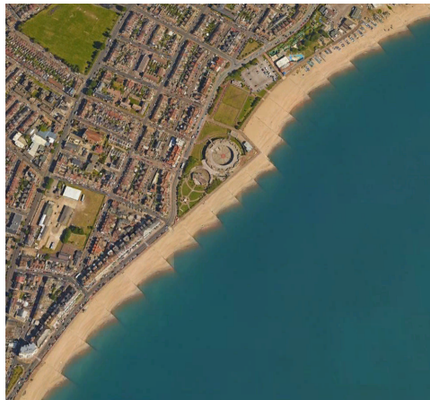
Figure G.2: Groynes with saw-tooth shaped beach
