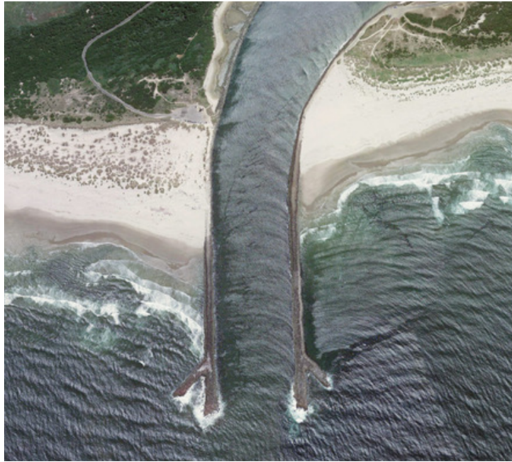
Figure G.4: Jetty for river-mouth stabilization
