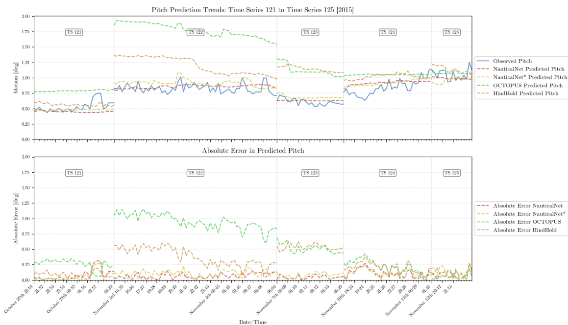
Figure 45: Comparing Pitch Predictions with Observed Motions: Time Series Analysis (121-125). This graph illustrates the effectiveness of ML-based approaches against (simulated) conventional approaches, highlighting the variations in nowcast and hindcast environmental data.
