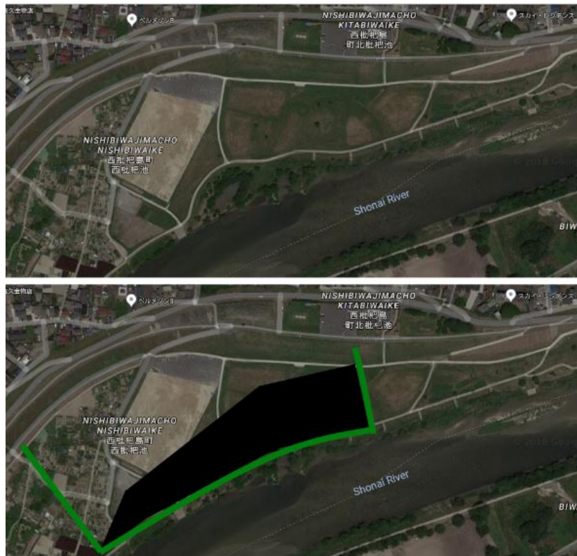
Figure AH.2: Area of building site outlet. Top: current situation; Bottom: Situation with building pit; Black: Future structure; Green: Temporary dike
