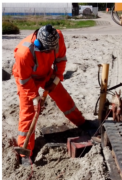
FIGURE C.7: Forming s-waves by hitting sideways on the steel box. Picture taken during the field test.
