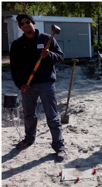
FIGURE C.6: Forming p-waves by hitting down on the steel plate. Picture taken during the field test.
