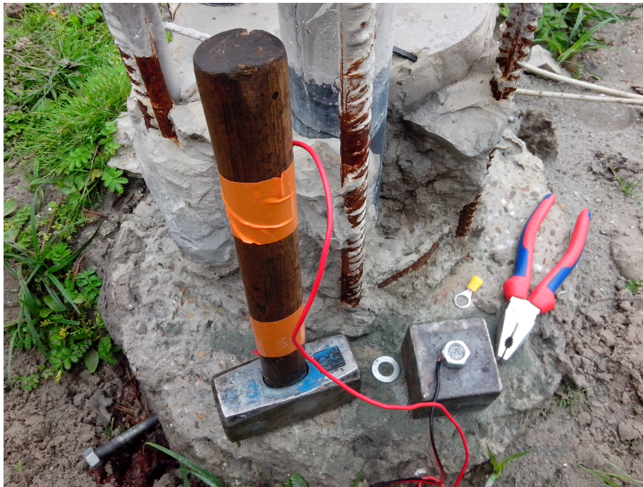
FIGURE C.5: Picture of the impact hammer used to introduce an impulse in the pile. To the left the stud can be seen on which the metal block is attached. Picture taken during the field test.
