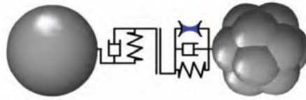
Figure 3.3: Visualization of contact between particles in DEM, including springs, dashpots, friction slider and cohesion bond[31]
