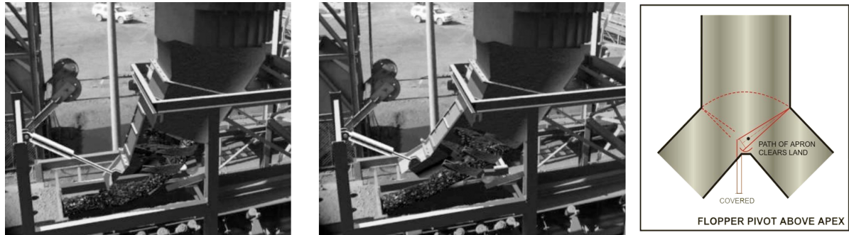
Figure 2.14: Chute redesign with adjustable spoon using hydraulic cylinder [23]. Maximum flow (left) and minimum flow position (middle). Flopper gate concept [10] (right)
