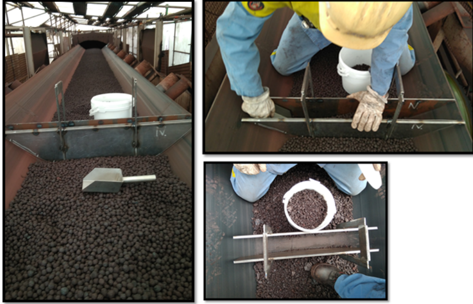
Figure 4.2: The sampling tools on the top belt, A317 (left), the process of sampling (top right) and a finished sample(bottom right)
