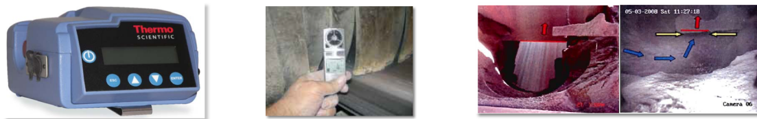
Figure 3.1: Personal Data Ram, PDR, measures dust in air (left) [30], Anemometer, measures air velocity (middle) [1], camera footage inside chute (right) [7]
