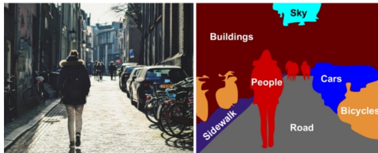
Figure 2.4: An example of image segmentation used in computer vision for self-driving cars.
