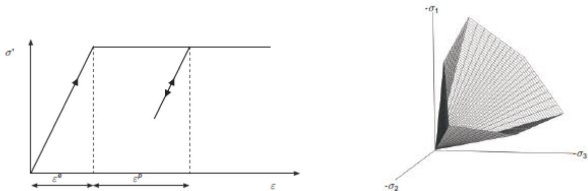
Figure 6 Stress-Strain relationship of a linear elastic perfectly plastic material (left) and the Mohr Coulomb yield surface in principal stress space (right) (Plaxis bv, 2017)
