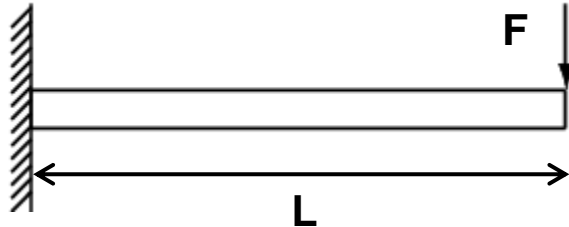
Figure 16 Cantilever beam with point load F
