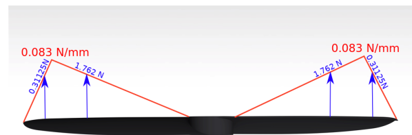
Figure 8.13: Approximated aerodynamic forces on propeller
