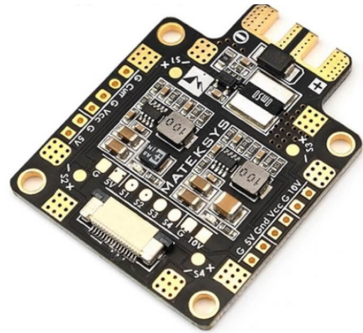
Figure 9.11: Similar PDB used for drone design [84]
