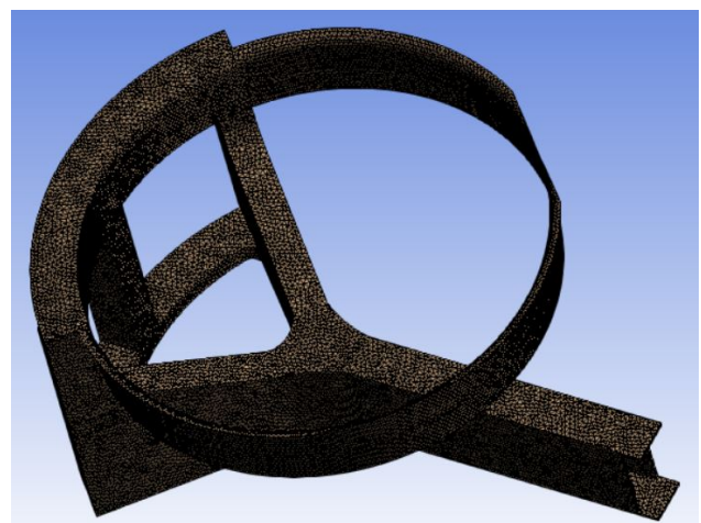
Figure 12.19: Fine meshing with tetrahedron elements with side of 0.5 mm
