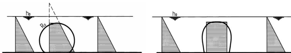
Figure 7: Difference between water filled (L) and air filled (R) system[4]
