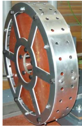
Figure 5.9: Photo of prototype axial flux PM generator after manufacture and assembly.
