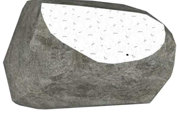
Figure 3.4b: Aggregate with contact area (white pattern), and contact point (black dot)
