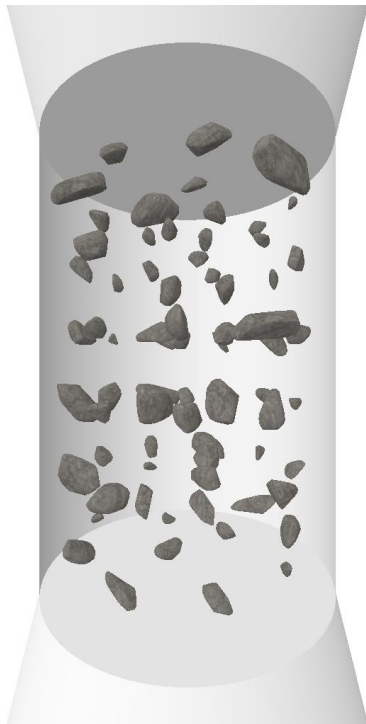
Figure 4.7a: Pre-placing with sufficient spacing
