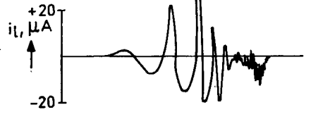
Fig. 13: Some typical interferences on the localizer current due to an overflying aircraft (Ref. 12).
