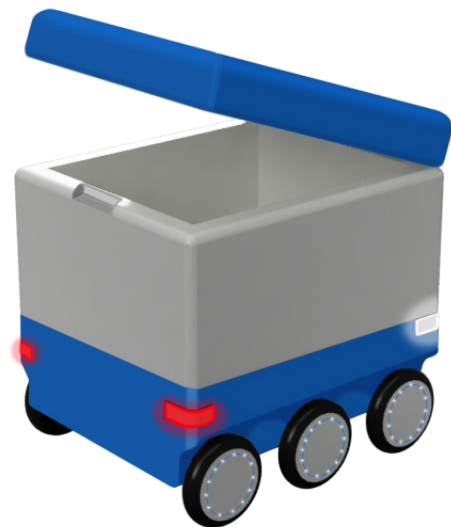
Figure 37, how the robot can be opened up from the backside.
