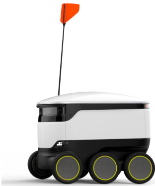
Figure 5, Starship Technologies delivery robot (Starship Technologies, n.d.).
