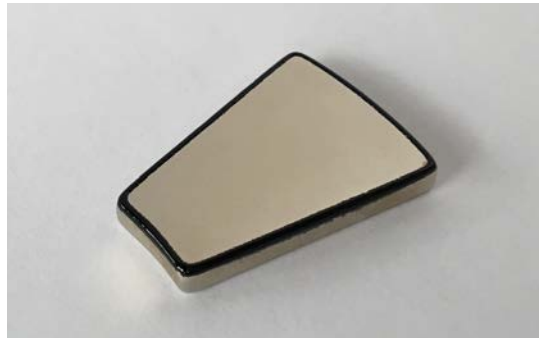
Figure 4.7: One magnet segment of 22.5^\circ with ferrofluid. The ferrofluid collects at the corners of the magnet and can seal a pocket of air, creating a planar bearing.
