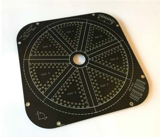
Figure 4.10: Final stator design: seven coils are embedded in a PCB.
