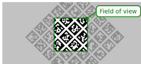
Figure 3.4: Field of view of the image sensor. Theoretically the field of view should be 2\sqrt{2} times as large as the size of one marker, to make sure one marker is always visible. For robustness, a field of view of four times one marker is selected.
