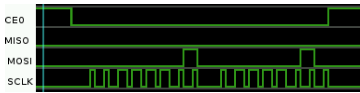
Figure I.2: SPI communication measured with piscope: sending out two bytes over SPI. First slave select 0 (CE0) is switch low to select slave 0, then the clock (SCLK) is enabled and is switched 8 times per byte. The value of MOSI determines what bit is sent each clock cycle. One byte consists of 8 bits. Binary 00000001 corresponds to a decimal 1 and 00000010 corresponds to a decimal 2.
