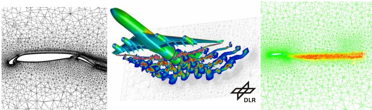
Figure 5 – Example of RANS data obtained for a high-lift wing configuration (AWIATOR, [41]).
