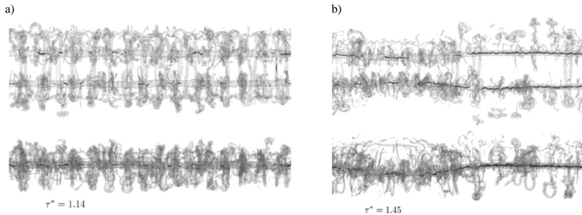
Figure 16 – Iso-vorticity surfaces from 3D LES simulations a) of the baseline configuration without oscillating ailerons at  $\tau^*=1.14$  [13]; b) of the baseline configuration with oscillating ailerons at  $\tau^*=1.45$  [30,31].
