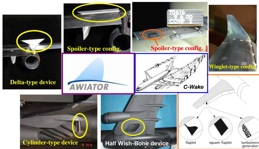
Figure 7 – Illustration of Wing add-on devices (C-Wake & AWIATOR projects).
