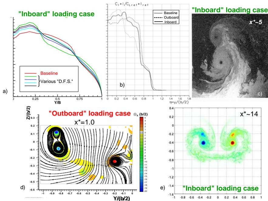
Figure 13 – Spanwise wing loading modifications for “Large transport aircraft-type model: a) computed load distribution [38]; b) load distribution deduced from measurements in the near-wake [24]; c) tomography of the wake flow field [4]; d) measured wake flow field at  $x^*=1$  [5,38]; e) computed wake flow field at  $x^*\sim 14$  [30,31].
