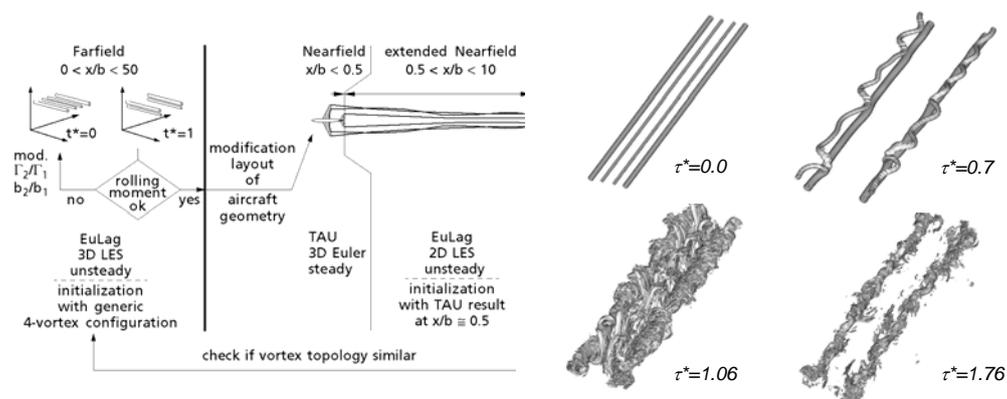
Figure 11 - Strategy for effective 4-vortex determination - left): numerical strategy; right): temporal development of iso-surfaces of vorticity for a given configuration [29].
