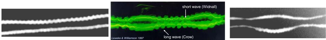
Figure 6 – Illustration of evidenced of short-wave and long-wave instabilities [2,25].
