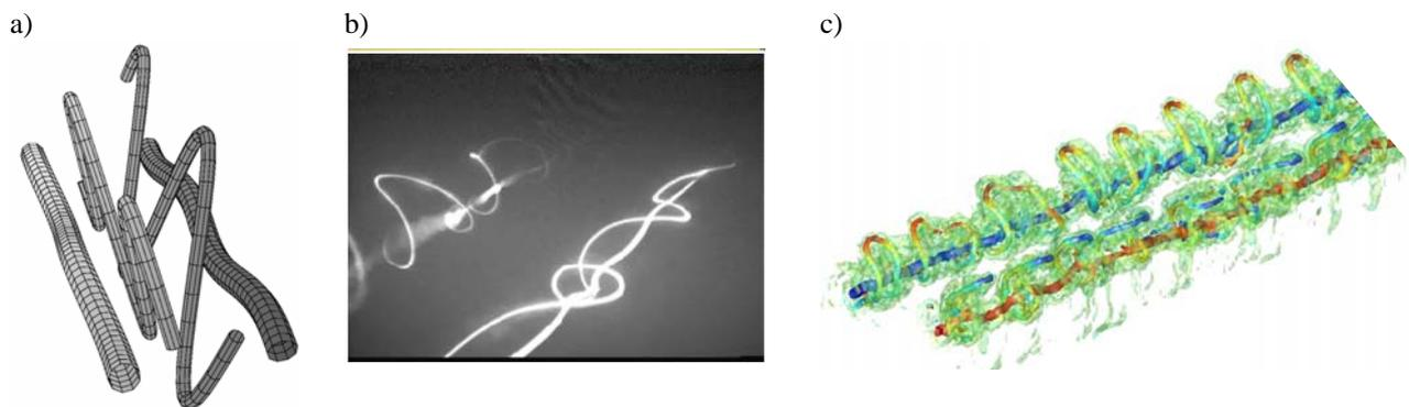
Figure 10 – Long wave perturbation in the wake of a 4-vortex system: a) linear stability theory [22]; b) Experiments [26]; c) iso-contours of vorticity at  $\tau^*=0.48$  for LES [30,31,36].
