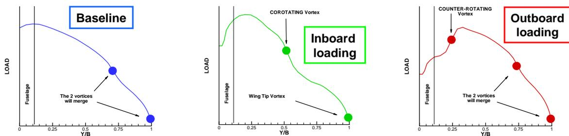
Figure 9 – Possible modifications of wing span load distribution ([38]).
