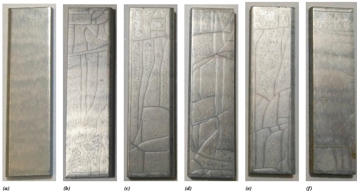
**Figure 4.10:** Comparison of pristine and spent SA-90-S stabilizer strips; evident is the high degree of surface cracking. a) Pristine and uncoated strip. b) Spent SA-90-DI-S. c) Spent SA-90-L-S. d) Spent SA-90-M-S. e) Spent SA-90-H-S. f) Spent SA-90-Cl-S.
