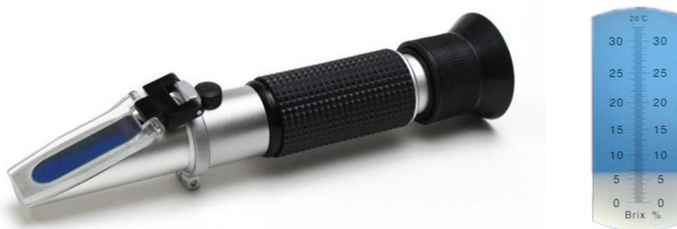
**Figure 2.8:** Refractometer used during all experiments in this research. The inset shows a typical reading in brix-%.
