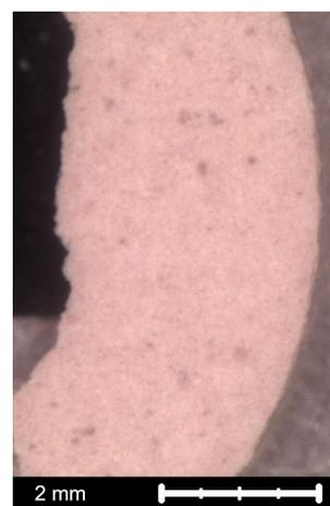
**Figure 3.9:** Magnified image of pristine  $\gamma\text{Al}$ -0.30 cercap showing dark spots on its surface.
