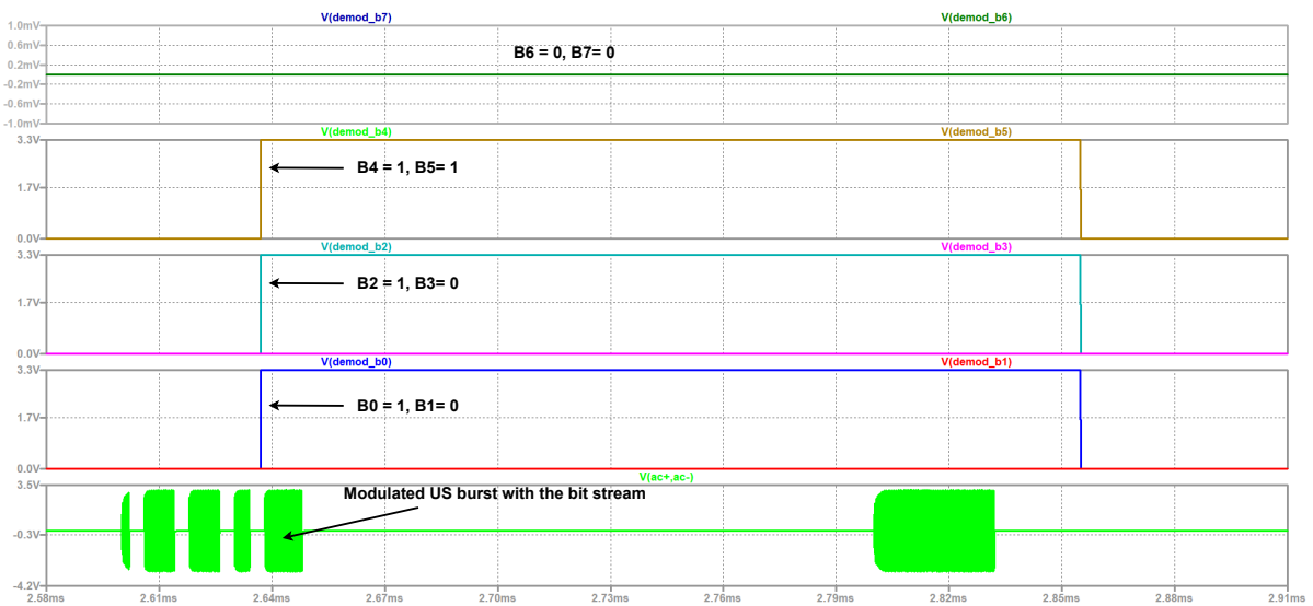
Figure 3.44: Waveform depicting the output of the 8-bit register stack and the decoded Forward Telemetry bitstream '10101100'.
