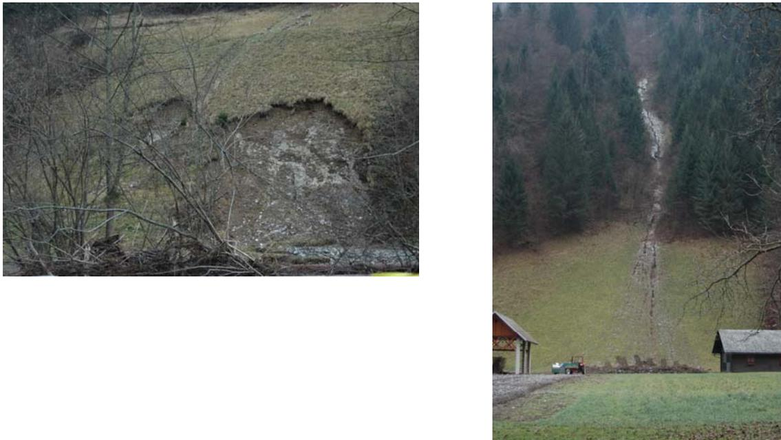
*Figure 4-4: Examples of a shallow slope failure and erosion rills observed on hill slopes after the September 2007 flood on the Selscica Sora basin (Slovenia)*
