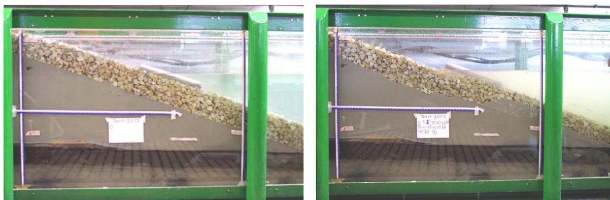
**Figure 1-2 Example of test 14 before the tests (left) and after 90 minutes of testing (right)**
