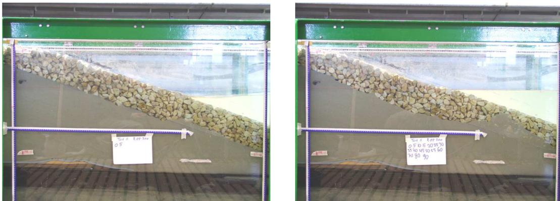
Figure 6-29 test 11 after 5 minutes (left) and after 90 minutes (right)
