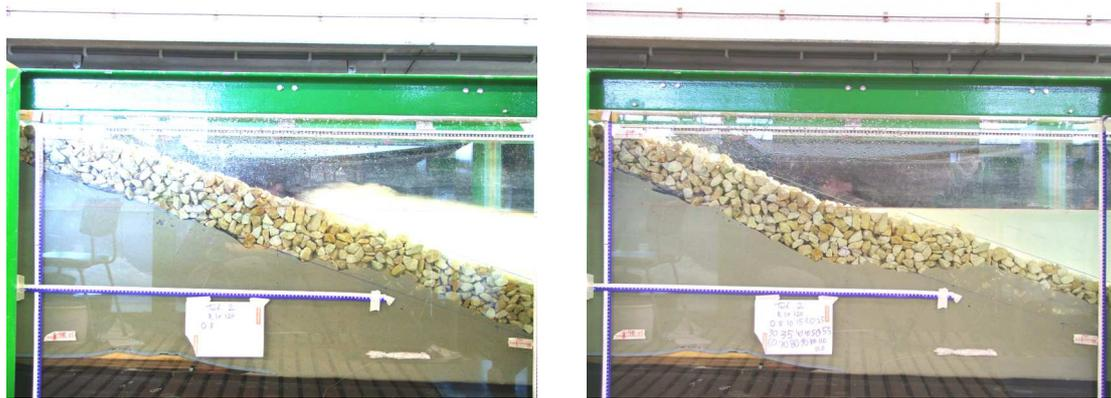
Figure 6-11 test 2 after 5 minutes (left) and after 120 minutes (right)
