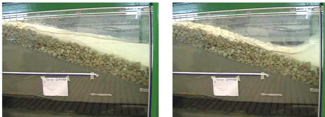
Figure 6-2 run-up (left) and rundown (right) of a large wave in test 10
