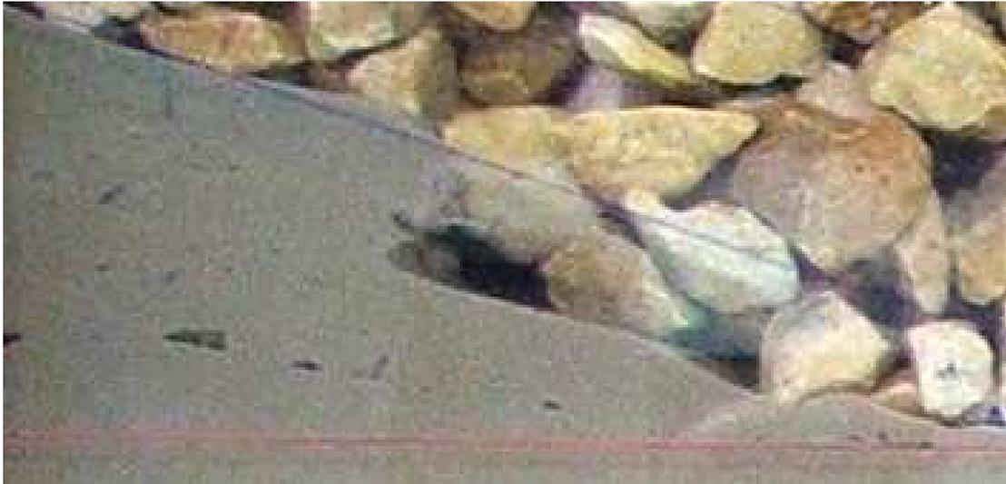
Figure 6-44 photo of the space under the mesh wire in test 3
