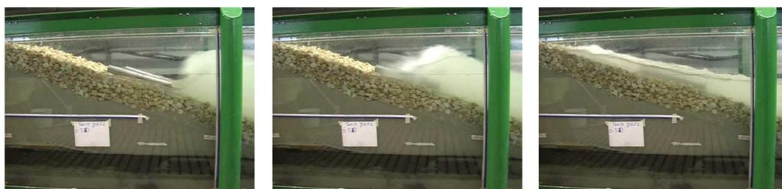
Figure 6-6 three stages of a breaking wave in test 14
