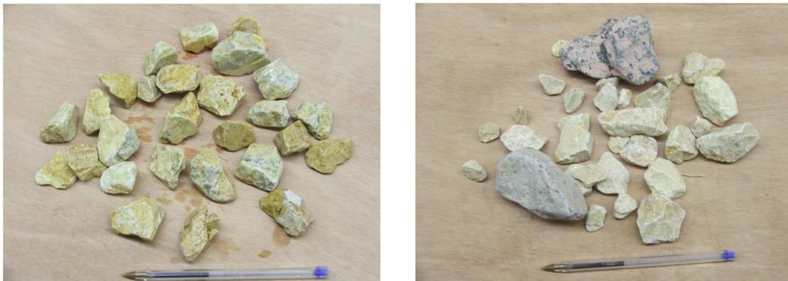
Figure 5-8 samples of the standard filter grading (left) and wide grading (right)
