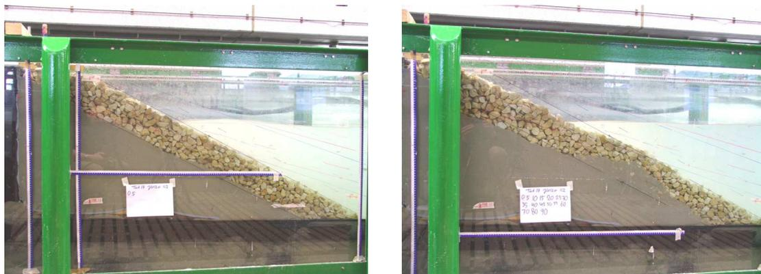
Figure 6-41 test 17 after 5 minutes (left) and after 90 minutes (right)
