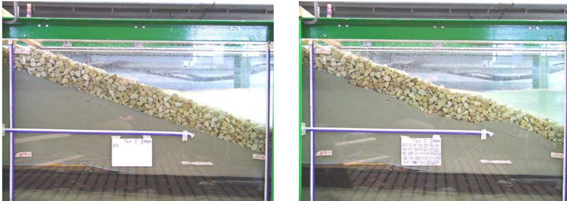
Figure 6-17 test 5 after 5 minutes (left) and after 600 minutes (right)
