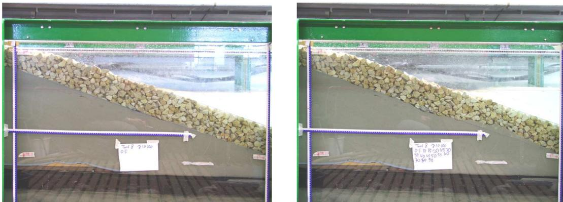
Figure 6-23 test 8 after 5 minutes (left) and after 90 minutes (right)
