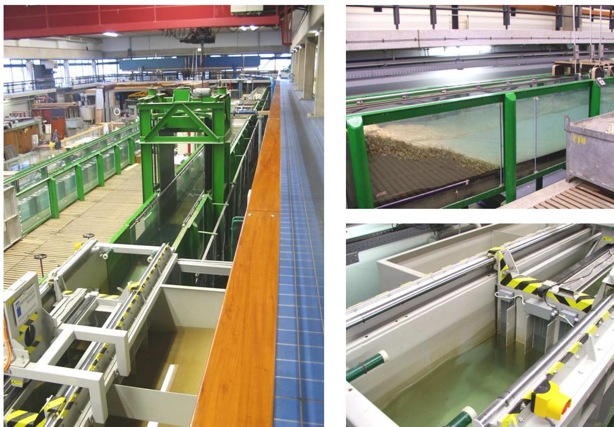
Figure 3-1 Small scale wave flume at the Fluid mechanics lab of TU Delft
