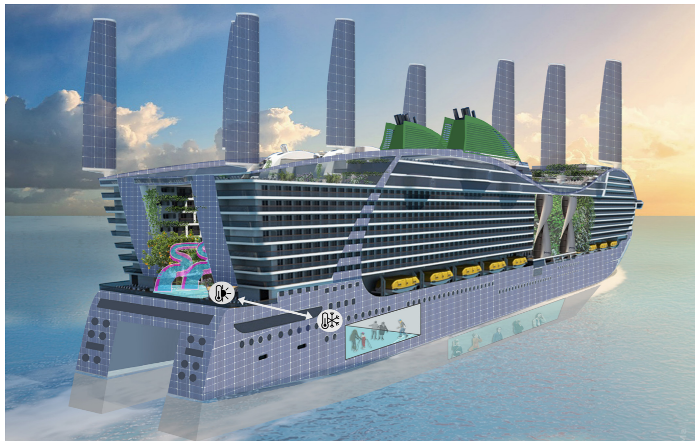
Figure 163: Future Cruise Ship with PV-film, sails with embedded PV-cells, wind turbine, algae, greenery, energy exchange principle, glass research lab.
