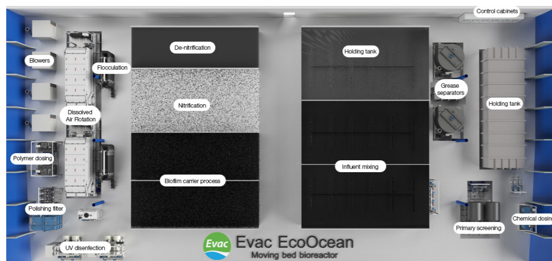
Figure 49: Process treatment system from EVAC Note. Reprinted from Evac. (2019).
