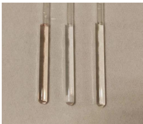
Figure S6.2 Photographic comparison of solutions of original complex (left, CB[8] = 0.6 mM, [ 1a 2+ ] = 1mM, [ 2b ] = 1mM), Nu1 (4 mM) added reacting for 8 hours (middle), and L-proline ( Nu2 , 4 mM) added reacting for 36 h (right).
