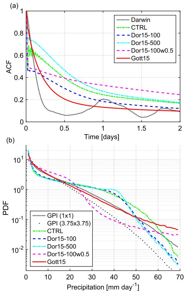
FIG. 4. (a) The autocorrelation function of  $M_b$  for Darwin observations and for SPEEDY ( $15^{\circ}\text{N}$ – $15^{\circ}\text{S}$ ) with CTRL, Dor15–100, Dor15–500, Dor15–100w0.5, and the Gott15 scheme. (b) The PDFs of the nonzero daily accumulated precipitation for GPI and for SPEEDY ( $15^{\circ}\text{N}$ – $15^{\circ}\text{S}$ ) with the same closures.
