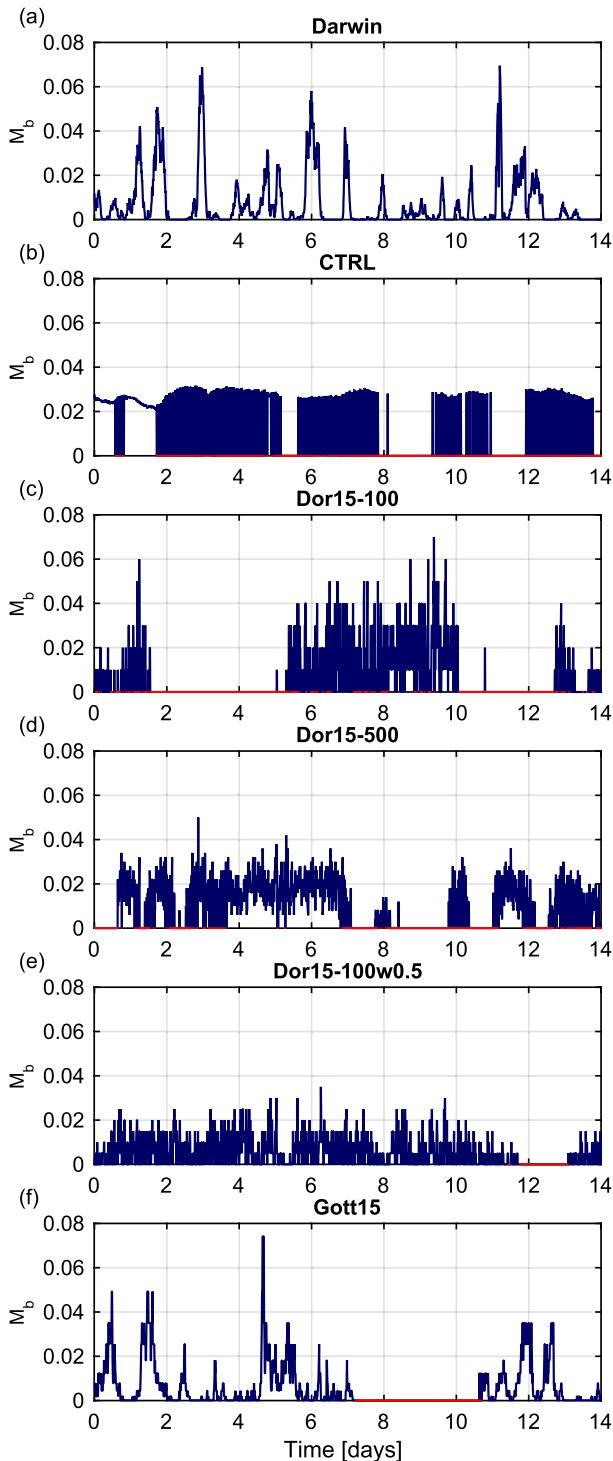
FIG. 2. Typical time series of  $M_b$  ( $\text{kg m}^{-2} \text{s}^{-1}$ ) (a) observed in Darwin ( $\sigma_c$  observations used as a proxy for  $M_b$ , assuming  $\rho w_c = 1 \text{ kg m}^{-2} \text{ s}^{-1}$ ) and produced by SPEEDY at  $13^\circ\text{S}$ ,  $130^\circ\text{E}$  for (b) CTRL, (c) Dor15-100, (d) Dor15-500, (e) Dor15-100w0.5, and (f) Gott15. An inactive trigger function is indicated by a red dot at the horizontal axis.
