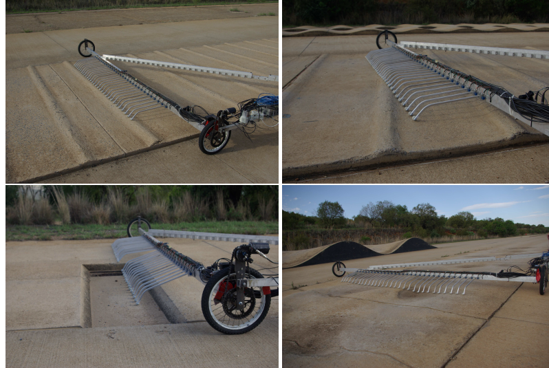
Figure 2.11: Each of the road profiles at the Gerotek testing facility being mapped for digital use.[2]
