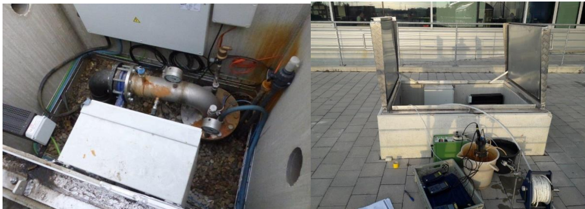
Figure 3: At the Belgian site, continuous temperature measurements (on the left a picture of an ATEs manhole, with an orange glass fiber on the right-hand corner) were combined with periodic elaborate geochemical assessments (on the right a picture of field equipment in operation); © Deltares, Nanne Hoekstra & André Cinjee
