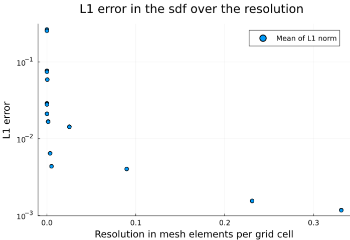
Figure 3.14: Mean L1 errors in the sdf of two interlocked links plotted over the resolution
