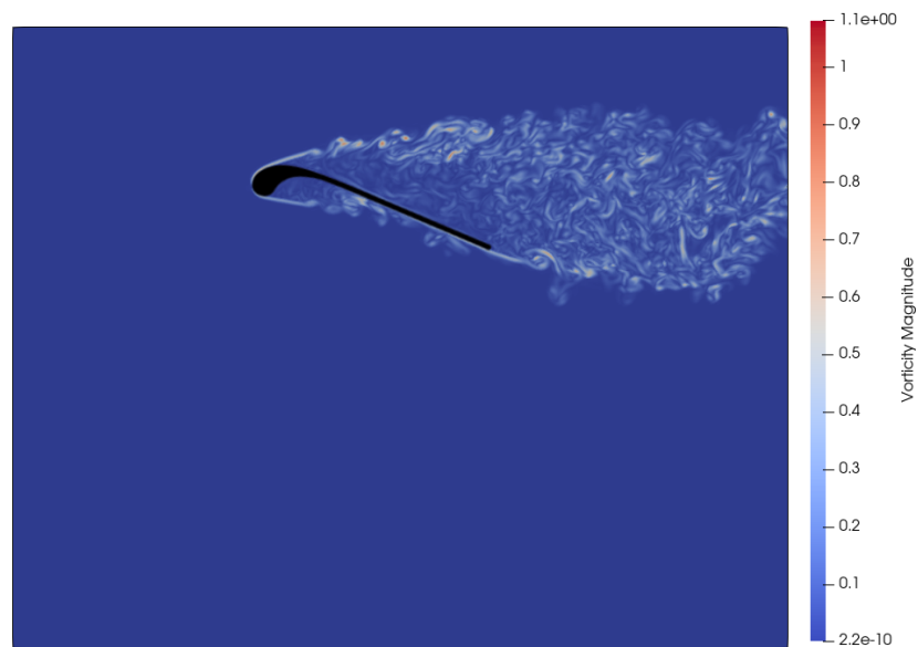
Figure 4.25: Vorticity magnitude in the wing symmetry plane for Re = 1 \times 10^5 and \alpha = 15^\circ
