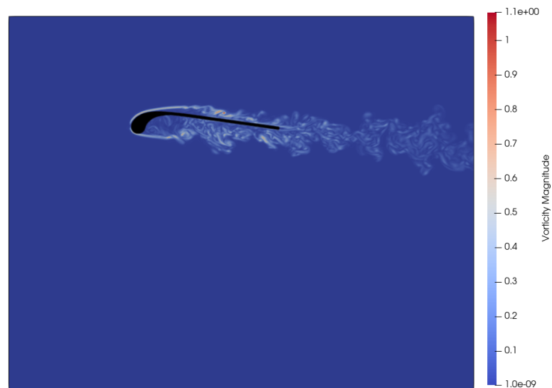
Figure 4.21: Vorticity magnitude in the wing symmetry plane for Re = 1 \times 10^5 and \alpha = 0^\circ
