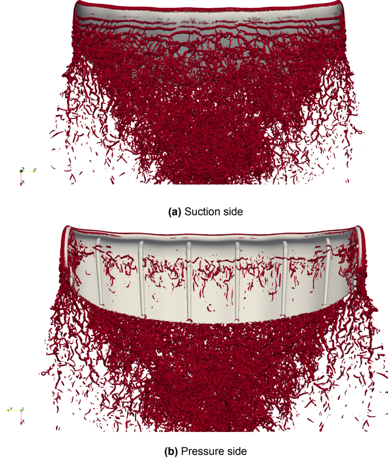
Figure 4.28: 3D representation of the Q-criterion iso-contours of Q_{crit} = 0.01 for Re = 1 \times 10^5 and \alpha = 20^\circ
