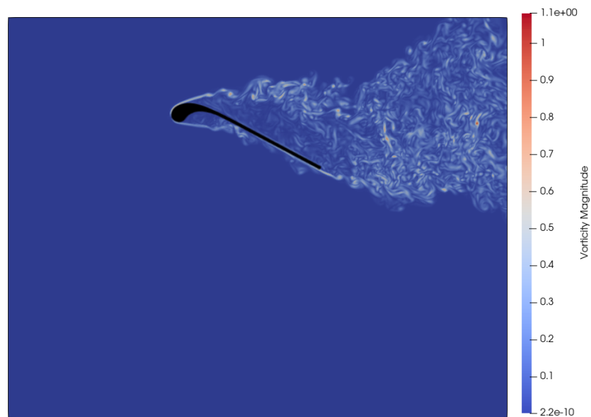
Figure 4.27: Vorticity magnitude in the wing symmetry plane for Re = 1 \times 10^5 and \alpha = 20^\circ
