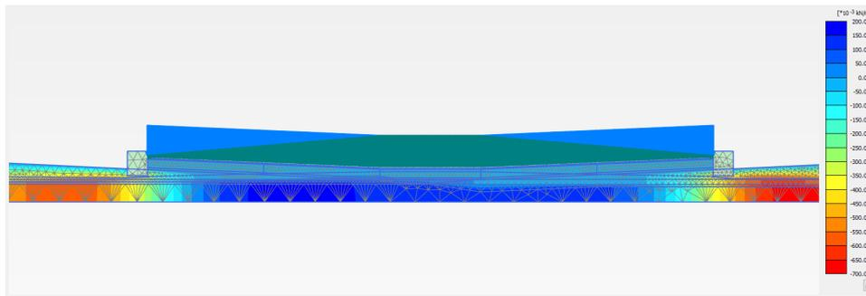
**Figure 6.34:** Excess pore water pressure distribution under the trough of the tide
