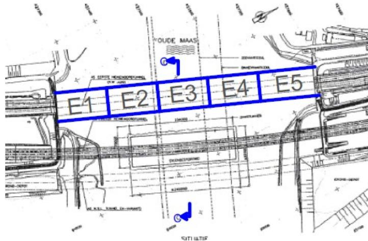
Figure 4.4: The plane view of Heinenoord tunnel
