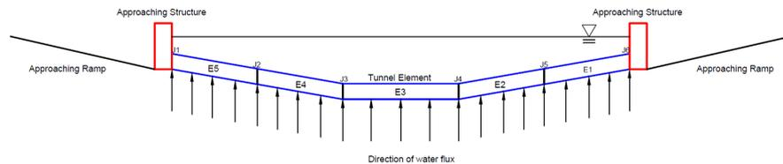
Figure 5.16: Location of immersion joint in Heinenoord tunnel
