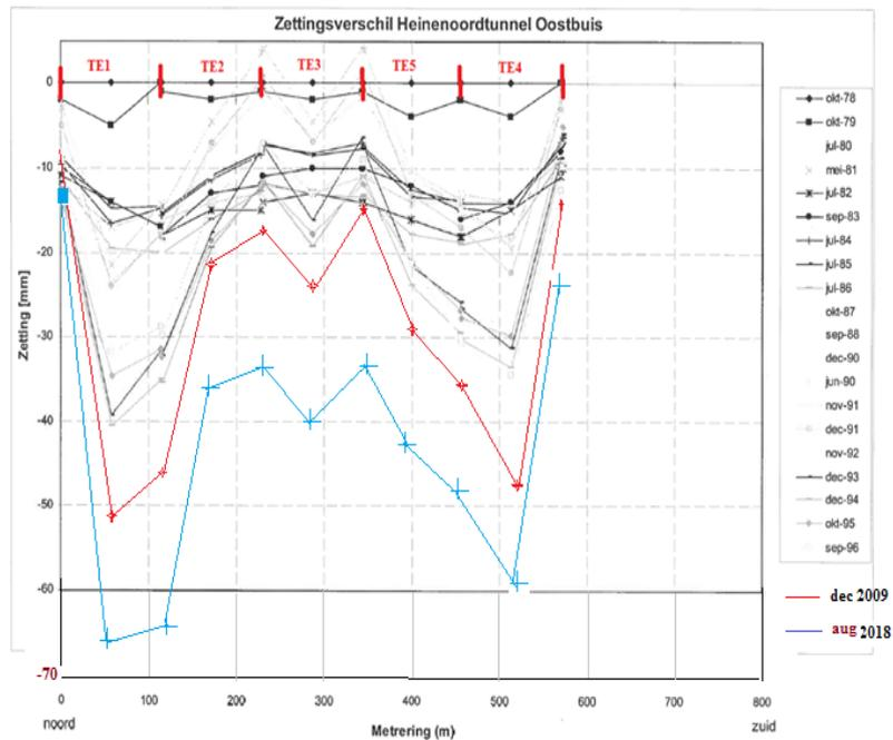
Figure 1.2: The settlement of Heinenoordtunnel (West tube) across 40 years of operation
