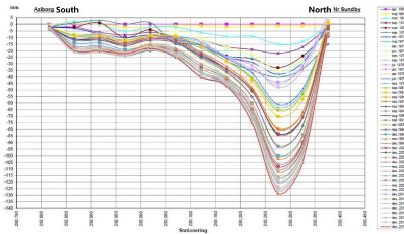
Figure 2.4: Long term Settlement of Limjford Tunnel
