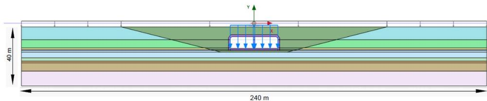
**Figure 4.3:** The input domain in the Plaxis model
