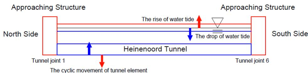
**Figure 1.5:** The cyclic movement of Heinenoordtunnel to tide variation
