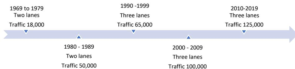
**Figure 4.18:** Traffic arrangement of Heinenoord tunnel during operation
