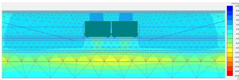
**Figure 5.10:** Settlement under average water level
