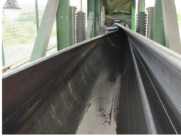
Figure 2.2: Folding belt from flat shape into a pipe shape (Image courtesy of Specialty Welding & Fabricating of New York, Inc.)
