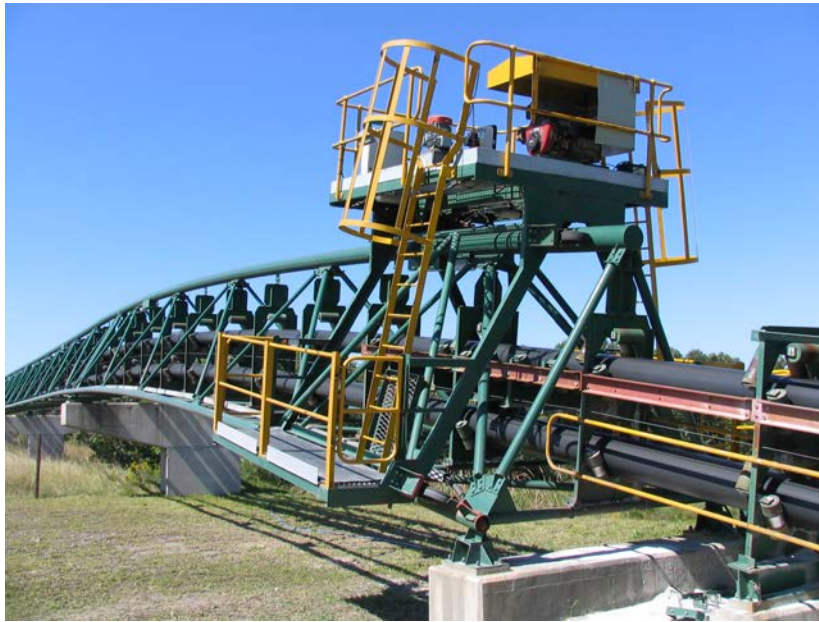
Figure 2.10: Triangular gantry (Image courtesy of CKit Engineering (Pty) Ltd. [29]).
