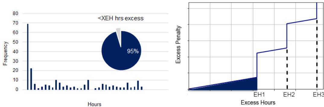
Figure 7.7: Left: Histogram and piechart of the excess hours, Right: piecewise linear function for excess penalty, the highlighted section indicates excess hours smaller than XEH hours
