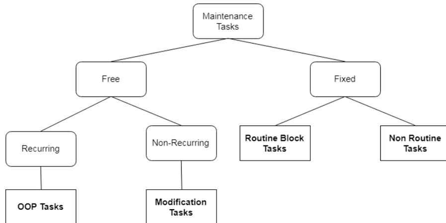
Figure 4.1: The distinction of two groups of maintenance tasks in the model: recurring and non recurring tasks
