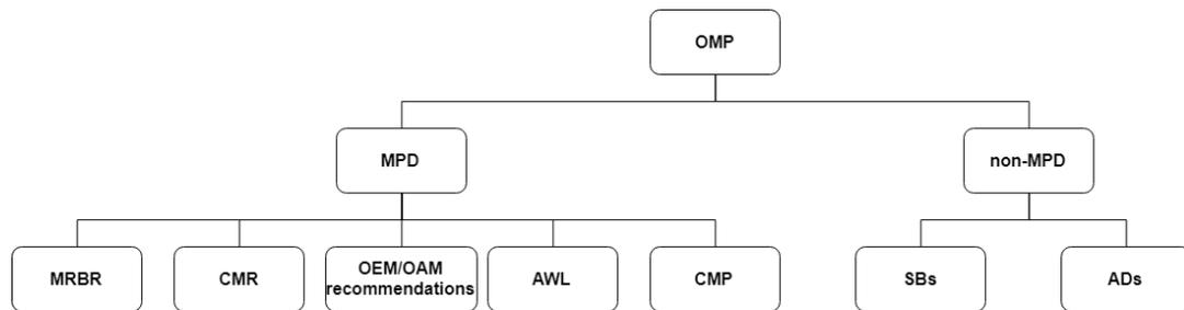
Figure 3.4: Schematic overview of the origins of tasks contained in an Operator's Maintenance Program
