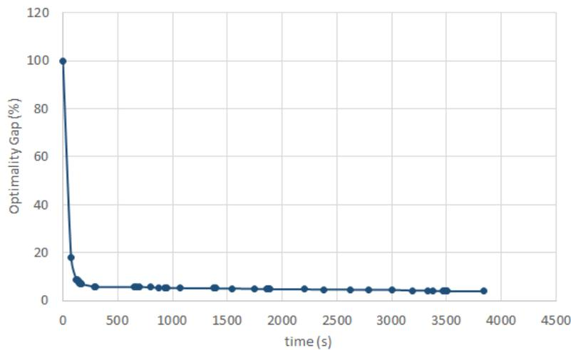
Figure 7.9: Convergence rate shown by the reduction of the optimality gap over time
