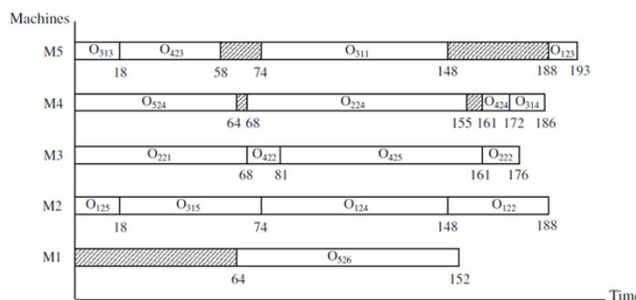
Figure 2.1: Example of one of the schedules of the FJSSP-FPP model of Ozguven et al. in which each of the jobs consisted of several operations (subtasks) which in turn had various optional sequences in which they could be executed. The allocation of the operations to the machines is optimized for minimum makespan [1]
