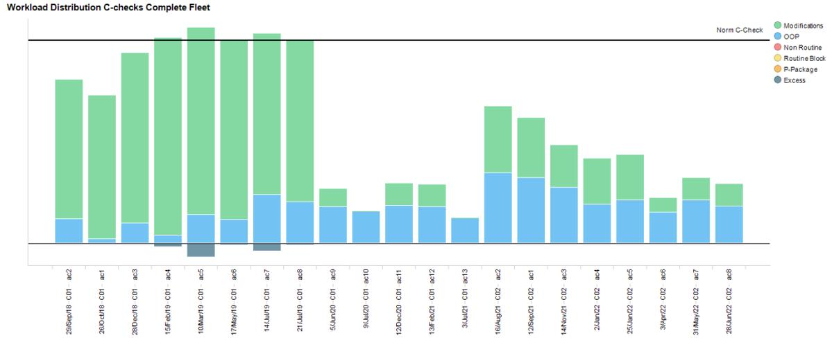
Figure 7.4: Workload distribution of the C-checks for the airline's wide-body fleet over a four year planning horizon. From top to bottom the bar segments are the allocated capacity in required labor hours of the modifications and OOP tasks. The excess hours are shown on the negative y-axis.
