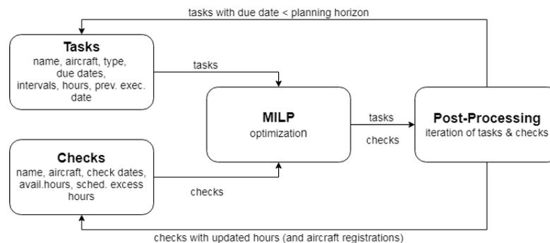
Figure 4.7: Schematic of the iterative solution technique built around the optimization run
