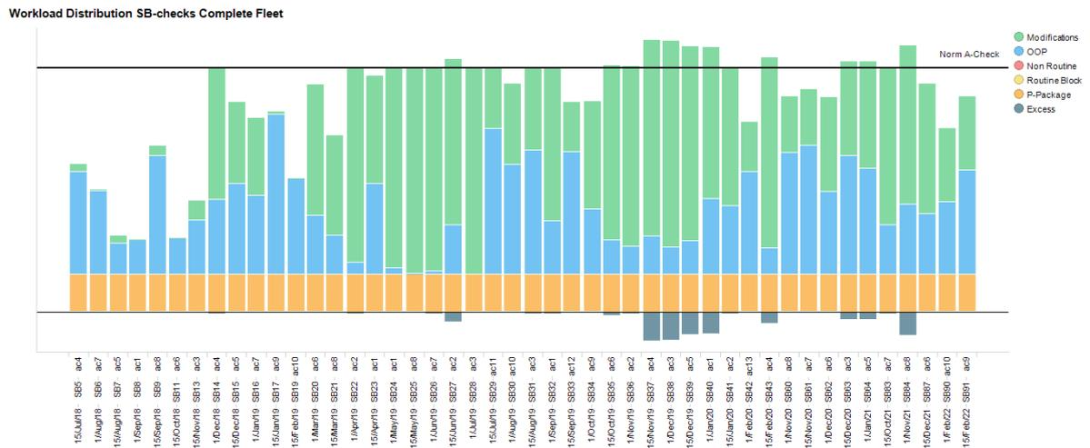
Figure 7.5: Workload distribution of the SB-checks for the airline's wide-body fleet over a four year planning horizon. From top to bottom the bar segments are the allocated capacity in required labor hours of the modifications, OOP tasks and P-packages. The excess hours are shown on the negative y-axis.
