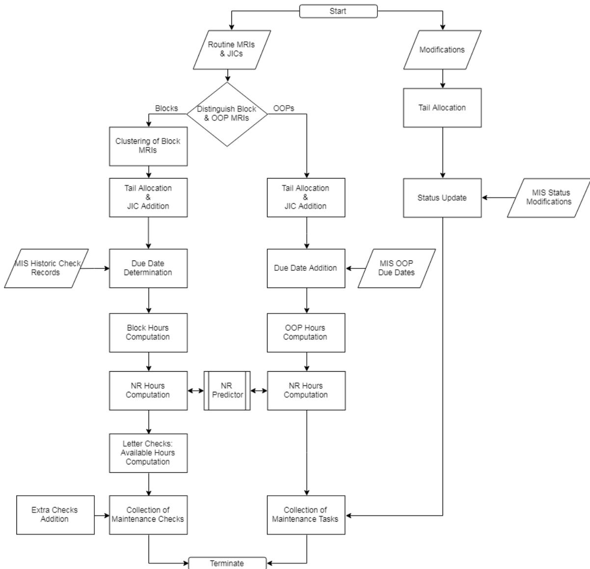
Figure A.1: Schematic overview of the data preparation process to prepare the optimization model inputs
