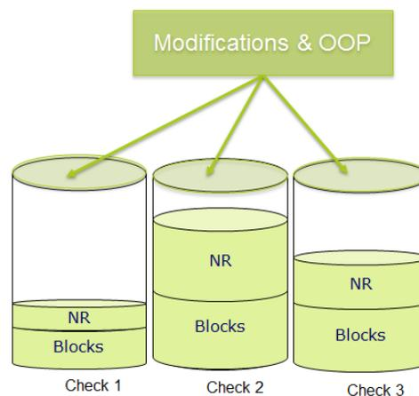
Figure 4.2: Schematic of the allocation of modification and OOP tasks to the maintenance checks, which have limited available capacity due to the routine block and non routine tasks that are fixed to the respective maintenance checks prior to the optimization
