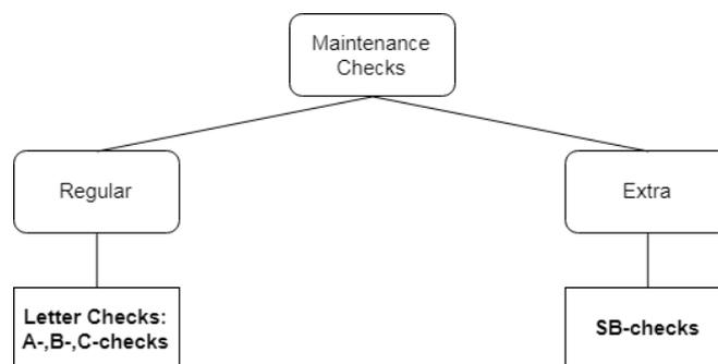
Figure 4.3: Schematic of the distinction between the regular, letter checks and extra, SB-checks
