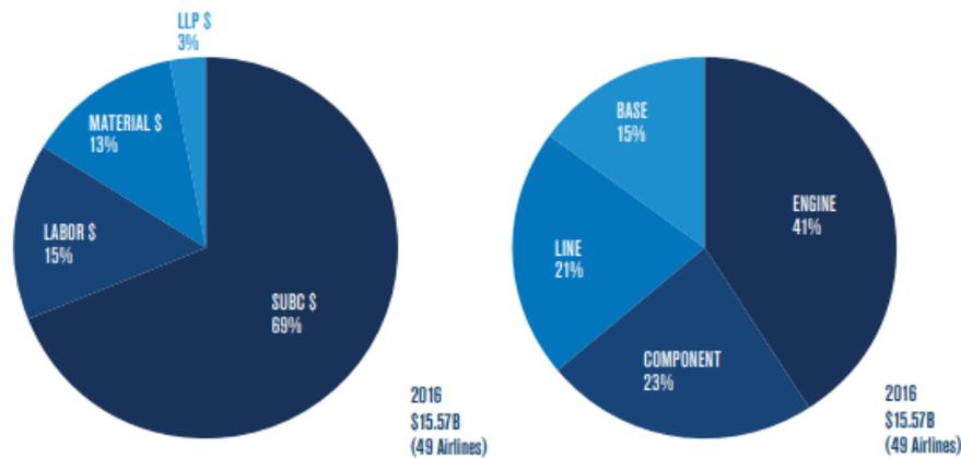
Figure 5.1: Breakdown of the primary direct maintenance costs (DMC) of aircraft maintenance (left) and breakdown of maintenance cost per segment (right) according to IATA's 2016 Airline Maintenance Costs Analysis [4]
