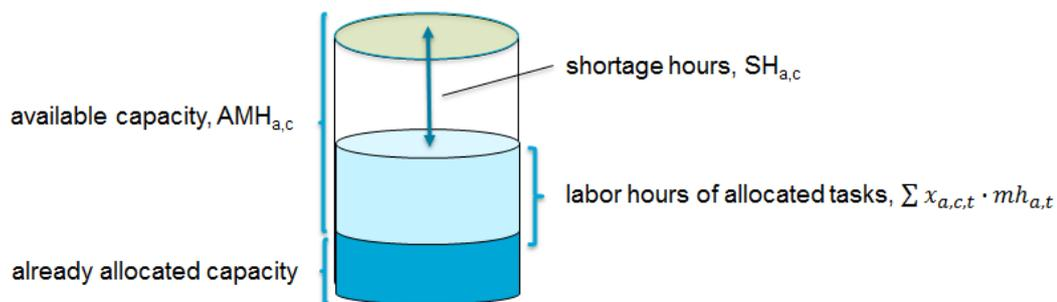
Figure 4.5: Illustration of the computation of the shortage hours as per the constraints in Equation 4.2
