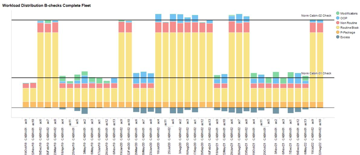
Figure 7.3: Workload distribution of the Cabin-checks for the the airline's wide-body fleet over a four year planning horizon. From top to bottom the bar segments are the allocated capacity in required labor hours of the modifications, OOP, non routine tasks, routine block tasks, p-packages. The excess hours are shown on the negative y-axis.
