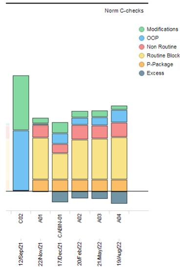
Figure 7.8: Overview of last year of the planning horizon of Aircraft 1; showing available capacity in the C02, followed by excess hours in the subsequent letter checks
