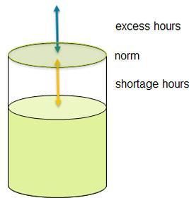
Figure 4.4: Illustration of the definition of shortage and excess hours with respect to the norm of the available resource capacity of a maintenance check
