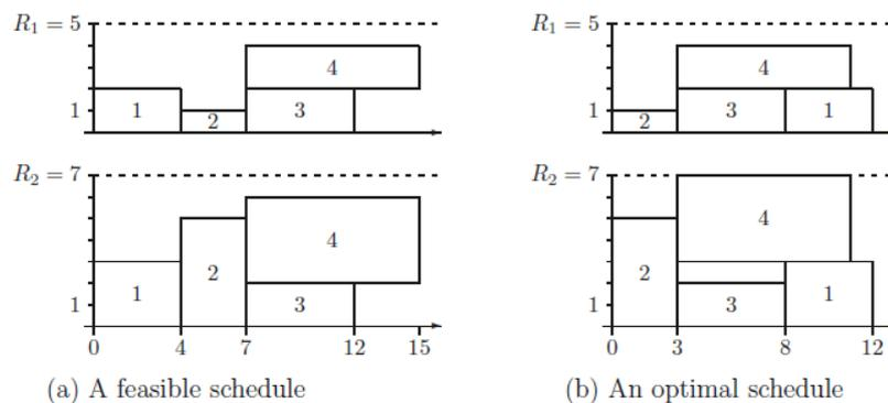
Figure 2.2: Example of a feasible (left) and optimal (right) schedule of an RCPSP consisting of four activities allocated over two resources [2]
