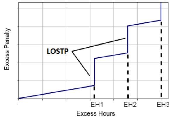
Figure 5.2: Piecewise linear function of the excess penalty versus excess hours as used in the model
