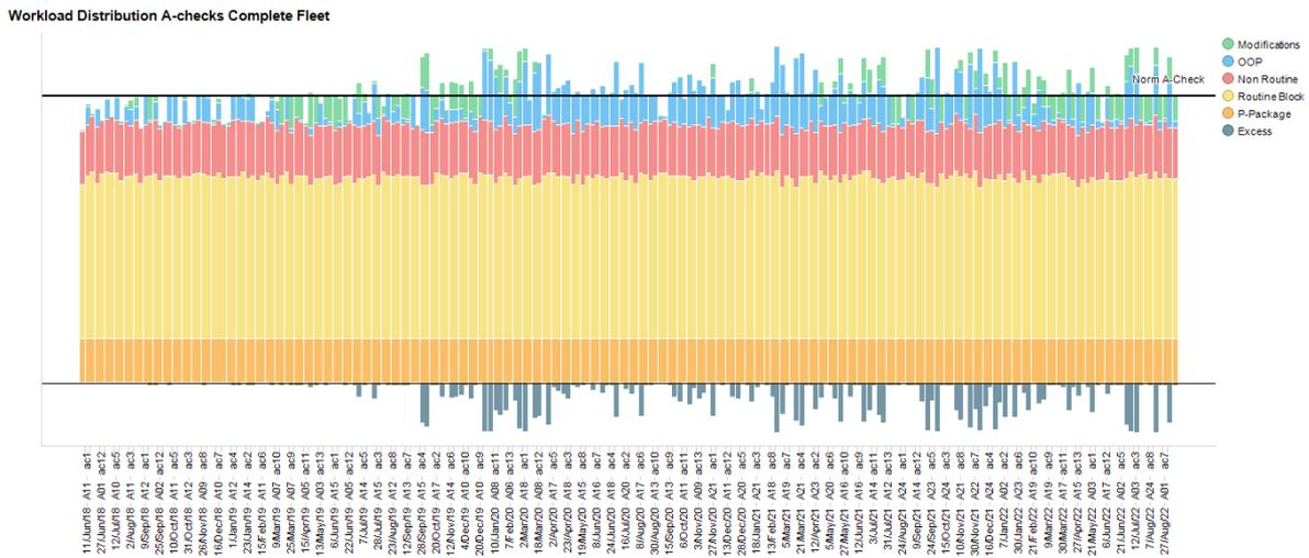
Figure 7.2: Workload distribution of the A-checks for the airline's wide-body fleet over a four year planning horizon. From top to bottom the bar segments are the allocated capacity in required labor hours of the modifications, OOP, non routine tasks, routine block tasks, p-packages. The excess hours are shown on the negative y-axis.
