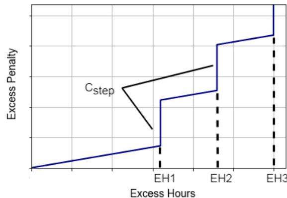
Figure 4.6: A simplified representation of the piecewise linear function that described the relation between the excess hours and excess penalty
