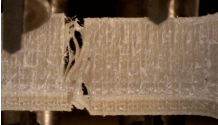
Figure D.20: Example of fracture in a A specimen (medium ABC) tested with the Zwick setup.
