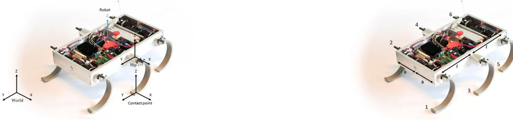
**Figure 4-4:** The coordinate frame assignments and the dimension of Zebro
