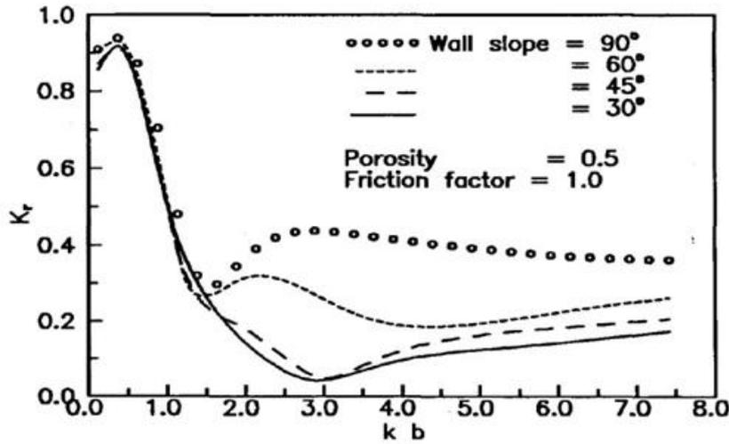
Fig. 9. Effect of wall slope on reflection coefficient.
