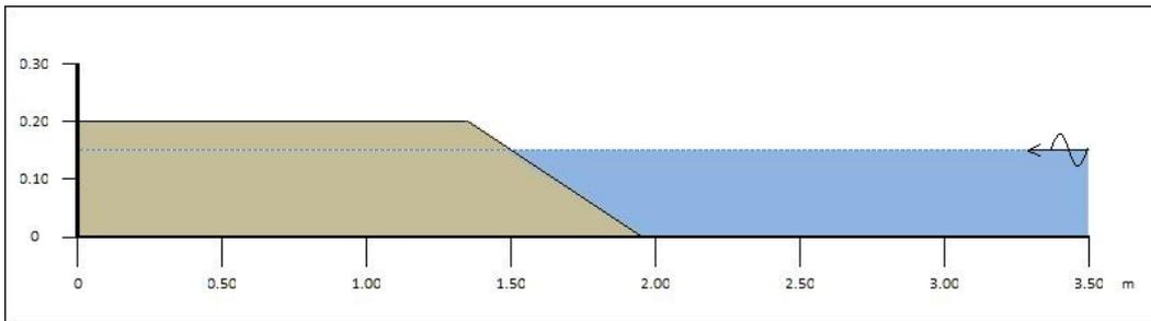
Figure 4.3: Lay-out B: Wave absorber with a 1:3 slope and length at SWL of 1.50 m
