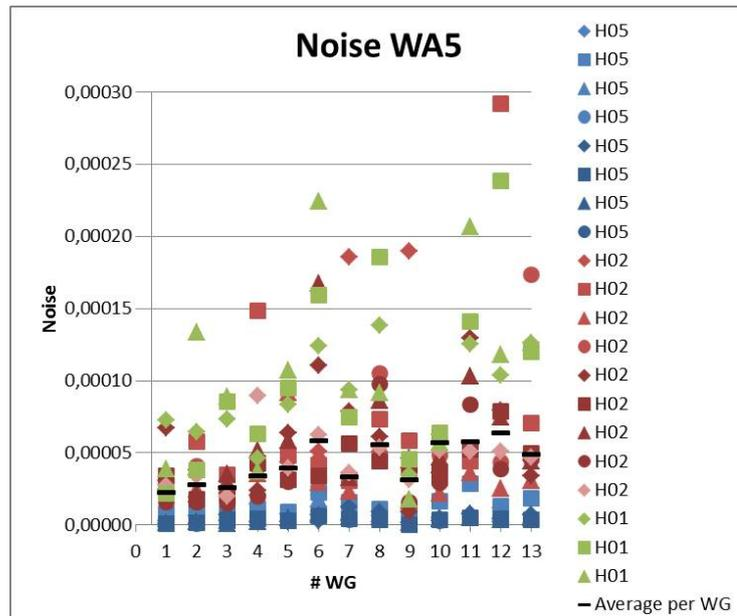
Figure 5.4: Distribution of results and average value per WG, for one wave absorber lay-out (all experiment runs)
