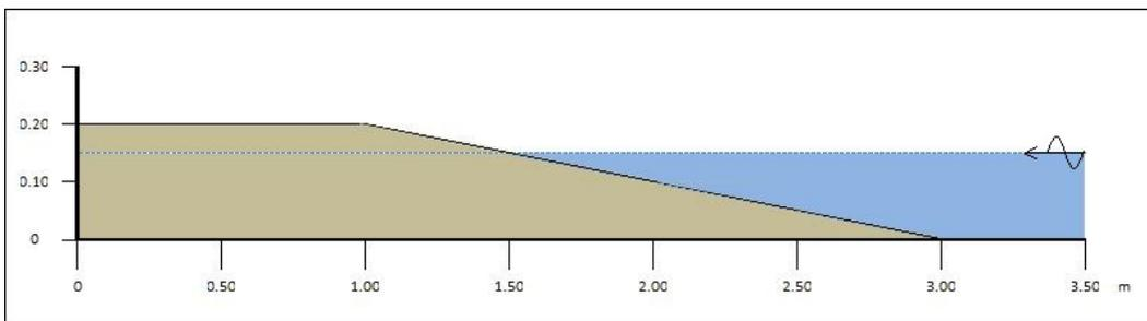
Figure 4.5: Lay-out D: Wave absorber with a 1:10 slope and length at SWL of 1.50 m
