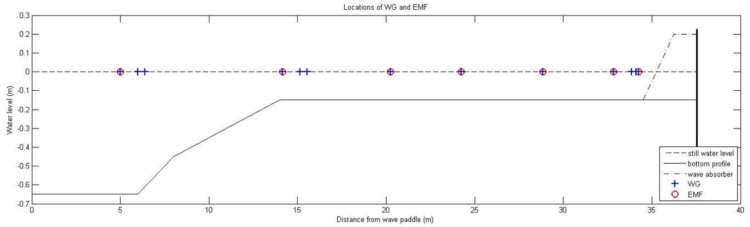
Figure 4.1: Locations of the wave gauges and EMF's along the flume
