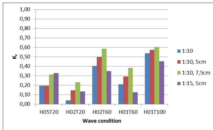
Figure 5.2: Comparison of the results for runs 8 to 10 (all with a 1:10 slope wave absorber, but different in toe) and run 11 (1:15 slope wave absorber), for implementation R3.  $K_r$  on the vertical axis
