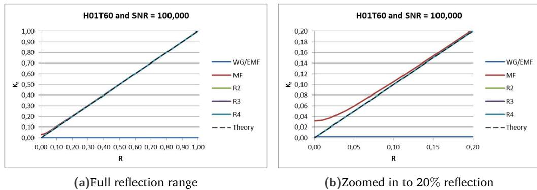
Figure 3.1:  $K_r$ -values as function of  $R$  for SNR = 100,000
