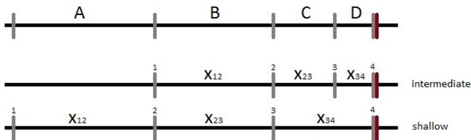
Figure B.3: Wave gauge spacing for intermediate and shallow water (dark grey indicates a WG, red indicates an EMF at shown positions)
