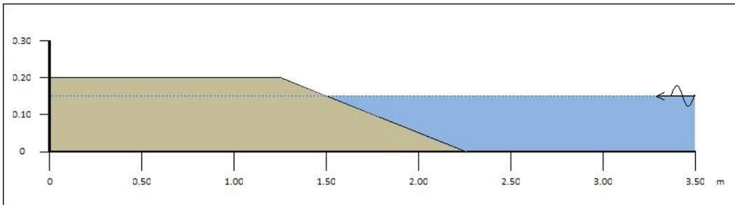
Figure 4.4: Lay-out C: Wave absorber with a 1:5 slope and length at SWL of 1.50 m
