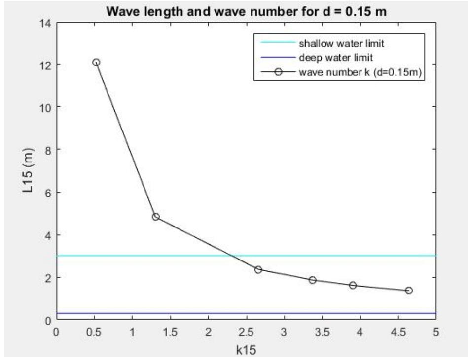
Figure B.1: Wave length and wave number for different wave periods for  $d = 0.15$  m
