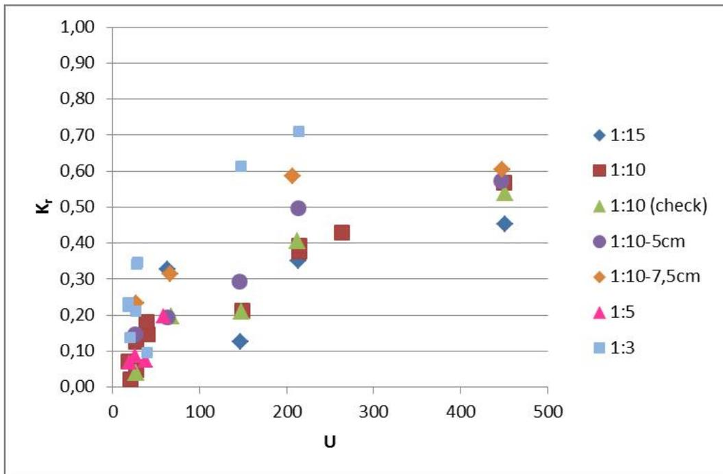
Figure 6.1: Reflection and Ursell number for all wave absorber lay-outs
