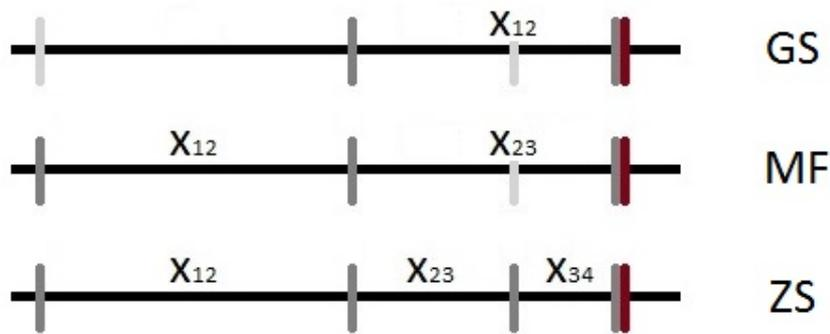
Figure B.2: Wave gauge spacing for intermediate and shallow water (dark grey indicates a WG, light grey indicates no WG, red indicates an EMF at shown positions)
