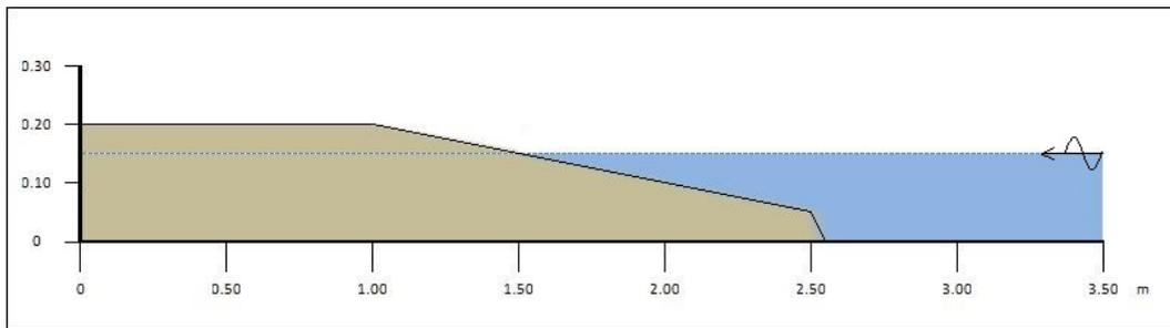
Figure 4.7: Lay-out F: Wave absorber with a 1:10 slope and length at SWL of 1.50 m, with a toe shortened at 0.05 m height
