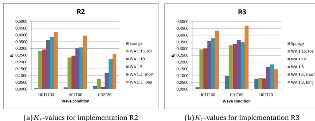
Figure 7.1:  $K_r$ -values per wave condition for a 50 m long sponge layer and various wave absorber lay-outs, for implementations R2 and R3, modelled with SWASH
