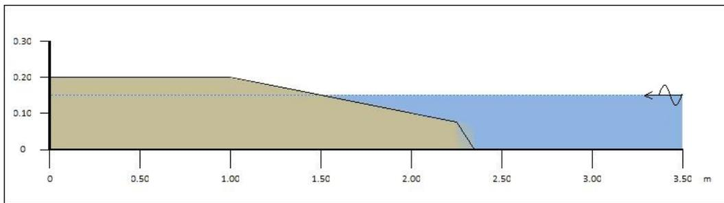
Figure 4.8: Lay-out G: Wave absorber with a 1:10 slope and length at SWL of 1.50 m, with a toe shortened at 0.075 m height
