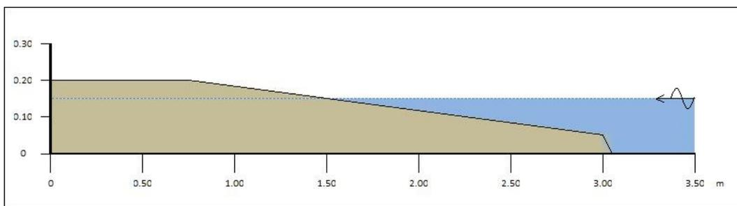
Figure 4.9: Lay-out H: Wave absorber with a 1:15 slope and length at SWL of 1.50 m, with a toe shortened at 0.05 m height
