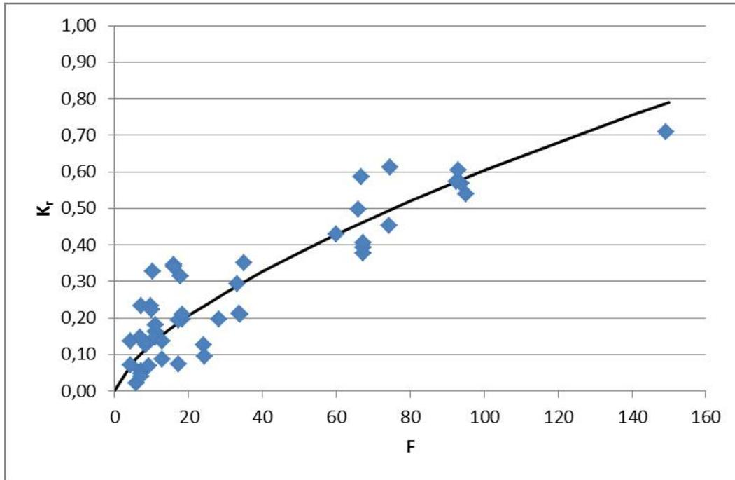
Figure 6.3: Reflection as function of factor  $F$  (Ursell number combined with slope), for all wave absorber lay-outs, compared to trend line (eq. (6.4))
