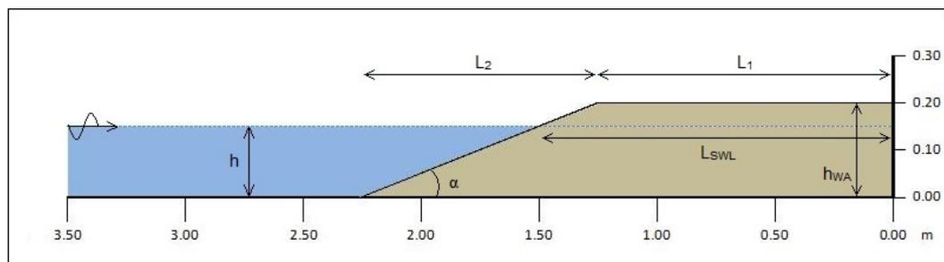
Figure 2.1: General wave absorber shape
