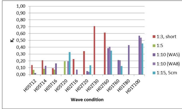
Figure 5.3: Comparison of the results for runs 6 (1:3 slope), 3 (1:5 slope), 5 and 8 (1:10 slope) and 11 (1:15 slope), for implementation R3.  $K_r$  on the vertical axis
