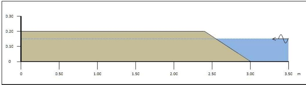
Figure 4.6: Lay-out E: Wave absorber with a 1:3 slope and bottom length of 3.00 m
