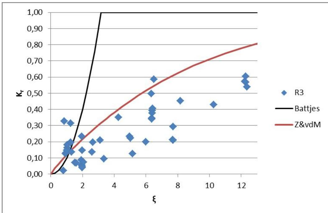
Figure 6.2: Reflection and Iribarren number for all wave absorber lay-outs, compared to theoretical lines of Battjes, (1974) and Zanuttigh and Van der Meer, (2006)
