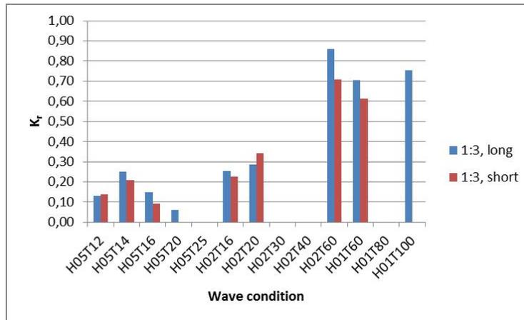
Figure 5.1: Comparison of the results for runs 4 and 6 (both with a 1:3 slope wave absorber, but different in length), for implementation R3.  $K_r$  on the vertical axis
