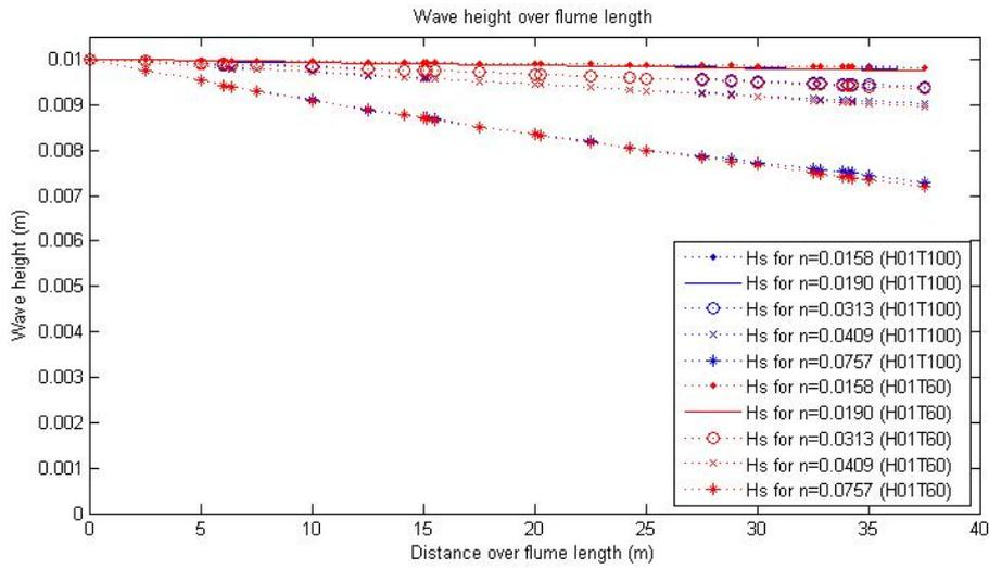
Figure 7.2: Decrease in wave height for two wave conditions over 37.5 m distance for various friction coefficient values
