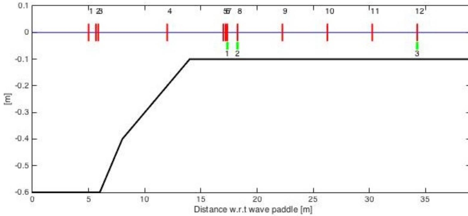
Figure C.2: Locations of the wave gauges and EMF's along the flume for the first series of experiments
