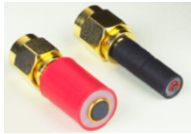
Figure 4.7: Probe tips: 4mm (red) 1.5mm (black)[6]
