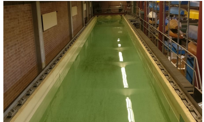
Fig. 3. Towing tank No.2, a wave maker facility of the Maritime & Transport Technology of TU Delft.
