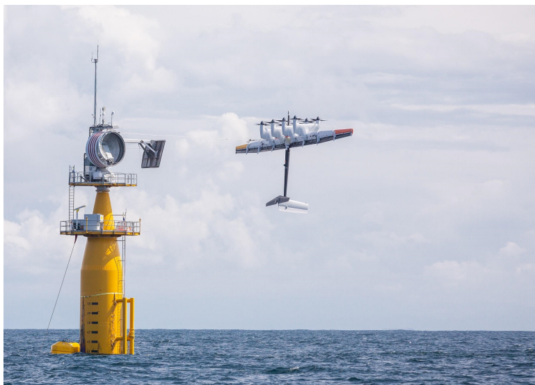
Figure 4: Makani AWE system being tested over the ocean. It is in powered flight mode next to its base station at the time this picture was taken[7].
