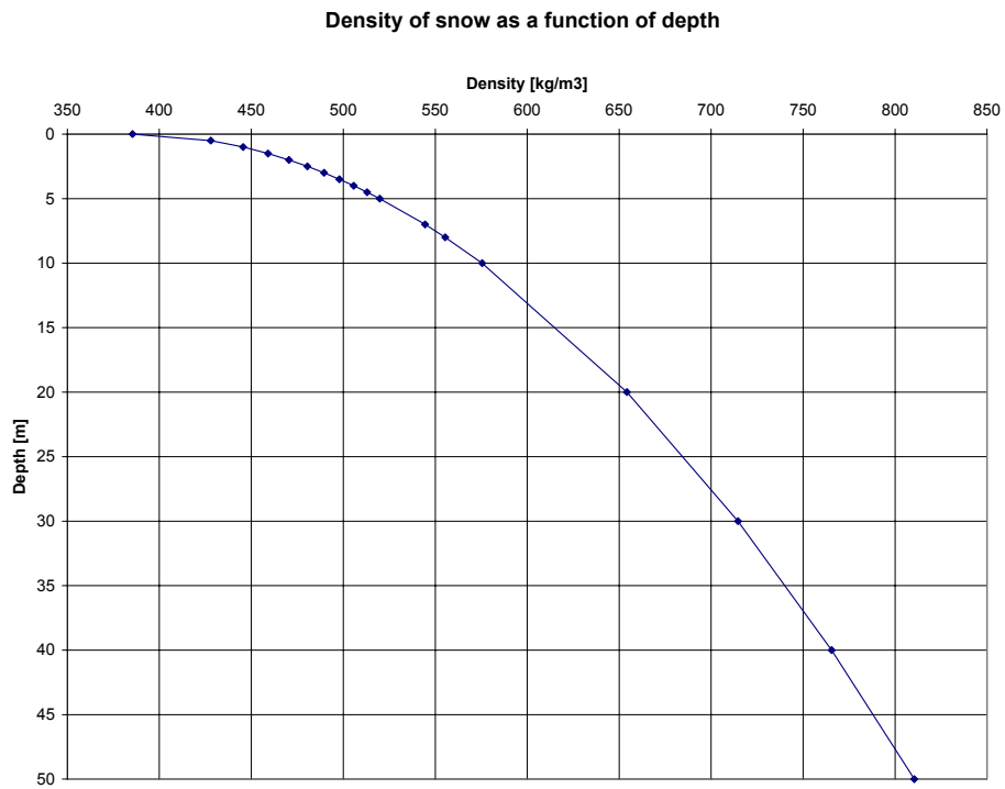
FIGURE 85: density of snow as a function of depth (source Enß [12])
