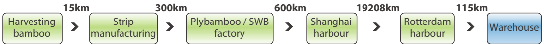
Figure 8. The production system for bamboo products used by MOSO International BV (cradle-to-warehouse-gate).
