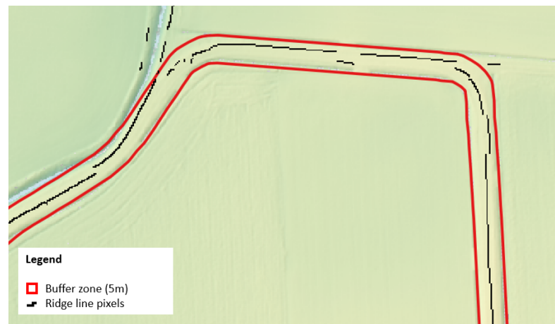
Figure 3.10: Buffer area with buffer distance of 5 m around manually drawn ridge line.
