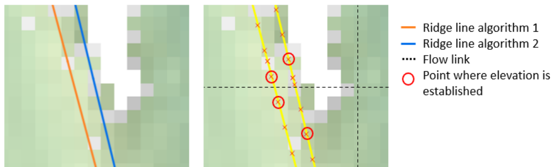
Figure 4.16: Determination of elevation. Points that are taken into account for the weighted average are indicated by red dots.
