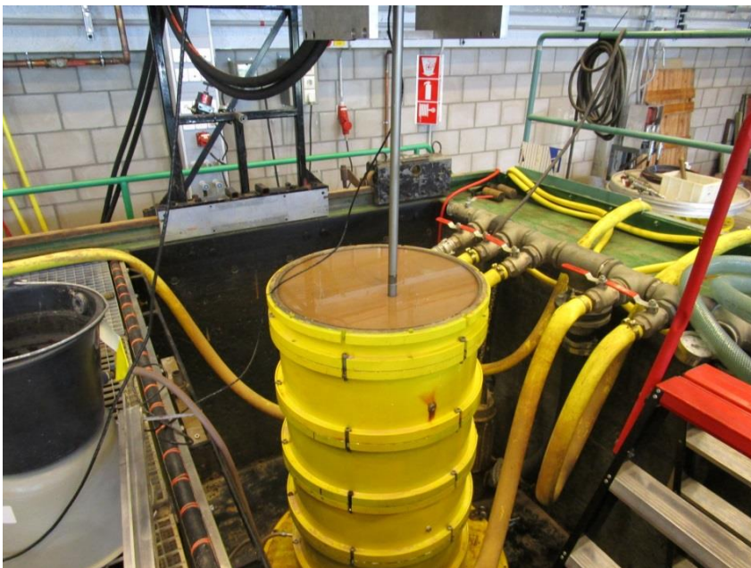
Figure 3: Test set-up (steel tank with sand sample, Test 7)
