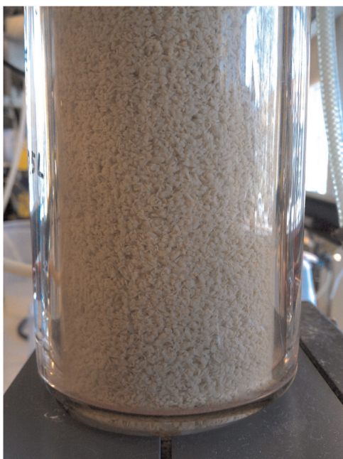
FIGURE 2 Impression of the 0.5–2 mm anaerobic granules in the reactor [Color figure can be viewed at wileyonlinelibrary.com ]
