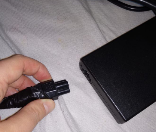
Fig 3.5.3 Disconnecting parts of a charger to avoid damaging the cord in their bag
