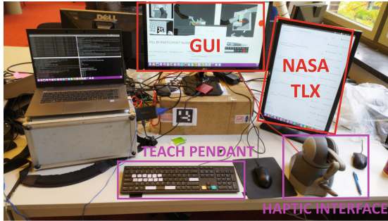
Fig. 3. Experiment setup with the teaching devices (purple), as well as graphical user interface (GUI) for visual feedback and a monitor to fill in the subjective questionnaire (NASA TLX).
