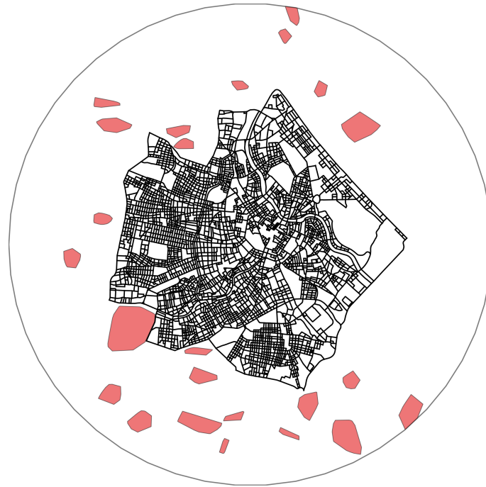
Figure 2. The Vienna airspace used in our system. The denser city centre is defined as constrained airspace, while the airspace around it is open airspace containing No Fly Zones (NFZ) areas. The overall airspace is a cylinder of an 8 km radius and 500 feet in height.
